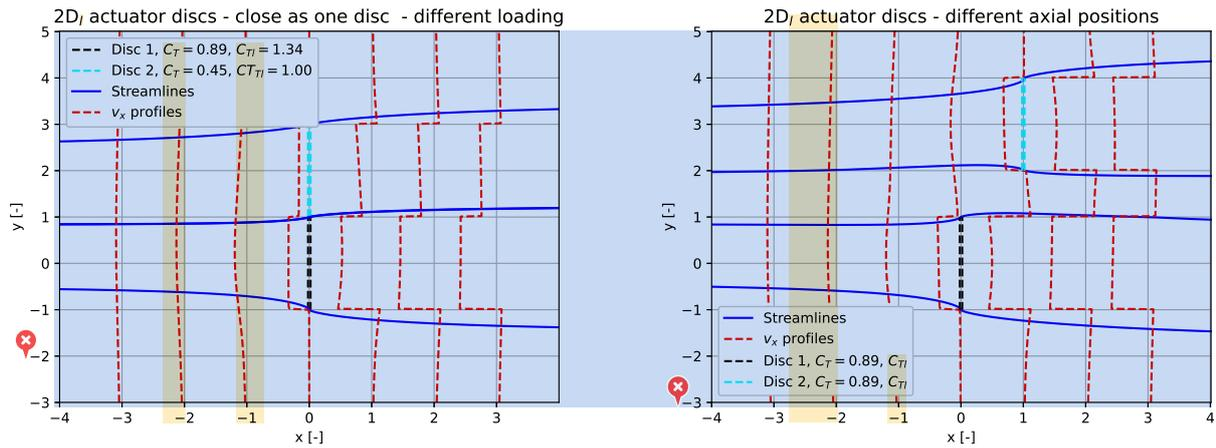
**Figure 4.** In the left graph we show the flow characteristics of two discs placed side by side so they just touch. The lower disc has the double loading of the upper disc. Enclosing streamlines for the two discs are shown together with  $v_x$  velocity profiles at different axial positions. To the right the same type of data are shown, however for the same loading on the two discs and with disc no. 2 shifted a distance of half the disc width in both  $x$  and  $y$  direction.
