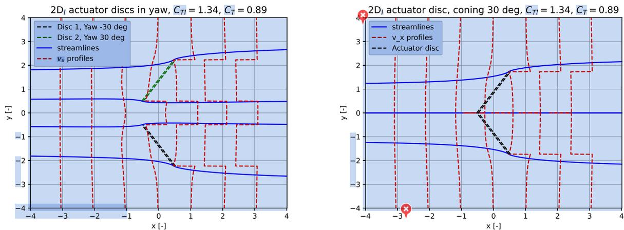
**Figure 11.** In the left graph we show two separated actuator discs with a yaw angle of  $30^\circ$  and  $-30^\circ$ , respectively. In the right graph they are moved towards each other so the edges just coincide and form one coned disc of  $30^\circ$  coning.
