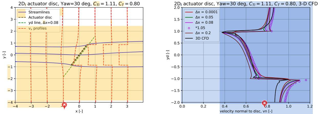
**Figure 8.** The left graph shows the enclosing streamlines of the yawed disc plus the streamline through the center of the disc for a yaw of  $30^\circ$ , respectively. Further  $v_x$  profiles are shown at three  $x$  positions. We show also the line  $yd$  along the disc in a distance of  $\Delta x = 0.08$  which is the line along which the normal velocity to the disc is shown in the right figure in comparison with 3-D CFD simulation of the AD.
