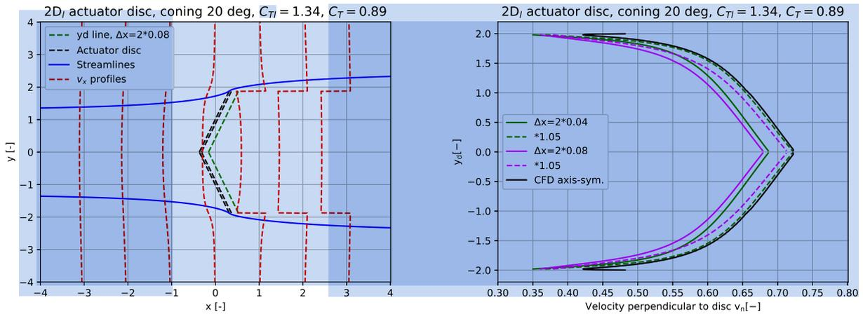
**Figure 12.** In the left graph we show the enclosing streamlines of a coned disc with  $20^\circ$  coning and a  $C_T = 0.89$ . In the same graph we also show the  $y_d$  line parallel with the two disc parts in a distance of  $\Delta x = 2 \cdot 0.08$  which are the lines along which we extract the velocities in the  $2D_l$  model for comparison with the CFD results in the right graph. However, the CFD velocities were extracted at the disc.
