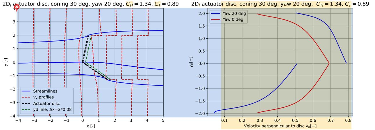
**Figure 16.** In the left graph we show the enclosing streamlines of a  $30^\circ$  coned disc with a yaw angle of  $20^\circ$  together with axial velocity profiles at different streamwise positions. In the graph to the right the normal velocity to the disc along the coned and yawed disc is shown in comparison with the velocities for an aligned coned disc.
