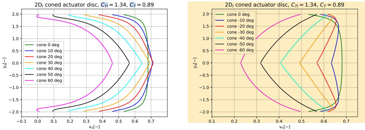
**Figure 15.** Simulated  $v_n$  distributions with the  $2D_l$  model for a range of positive cone angles in the graph to the left and for negative cone angled to the right.
