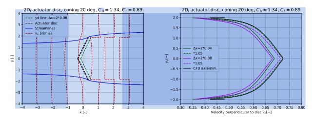
Figure 12. In the left graph we show the enclosing streamlines of a coned disc with  $20^{\circ}$  coning and a  $C_T = 0.89$ . In the same graph we also show the  $y_d$  line parallel with the two disc parts in a distance of  $\Delta x = 2 \cdot 0.08$  which are the lines along which we extract the velocities in the  $2D_l$  model for comparison with the CFD results in the right graph. However, the CFD velocities were extracted at the disc.
