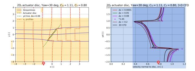
Figure 8. The left graph shows the enclosing streamlines of the yawed disc plus the streamline through the center of the disc for a yaw of  $30^{\circ}$ , respectively. Further  $v_x$  profiles are shown at three x positions. We show also the line yd along the disc in a distance of  $\Delta x = 0.08$ which is the line along which the normal velocity to the disc is shown in the right figure in comparison with 3-D CFD simulation of the AD.
