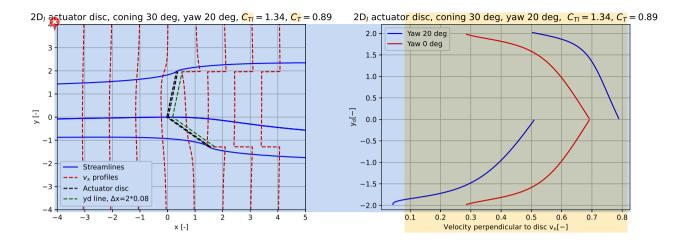
Figure 16. In the left graph we show the enclosing streamlines of a  $30^{\circ}$  coned disc with a yaw angle of  $20^{\circ}$  together with axial velocity profiles at different streamwise positions. In the graph to the right the normal velocity to the disc along the coned and yawed disc is shown in comparison withe the velocities for an aligned coned disc.
