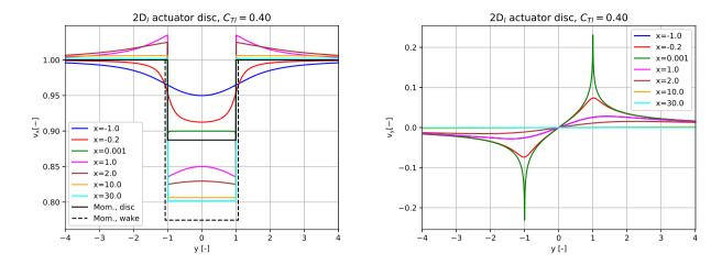
Figure 2. In the left graph the axial velocity component  $v_x$  is shown as function of the lateral coordinate y for different stream wise positions x from upstream the disc to far downstream in the wake for a thrust coefficient of 0.4. The velocity profiles for the momentum solution are also shown at the disc and in the far wake, respectively. In the right graph the lateral velocity component  $v_y$  is shown for the same positions.
