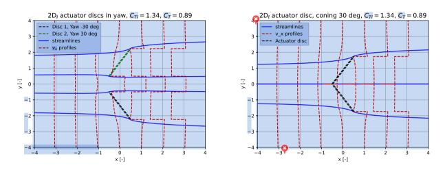
Figure 11. In the left graph we show two separated actuator discs with a yaw angle of  $30^{\circ}$  and  $-30^{\circ}$ , respectively. In the right graph they are moved towards each other so the edges just coincide and form one coned disc of  $30^{\circ}$  coning.
