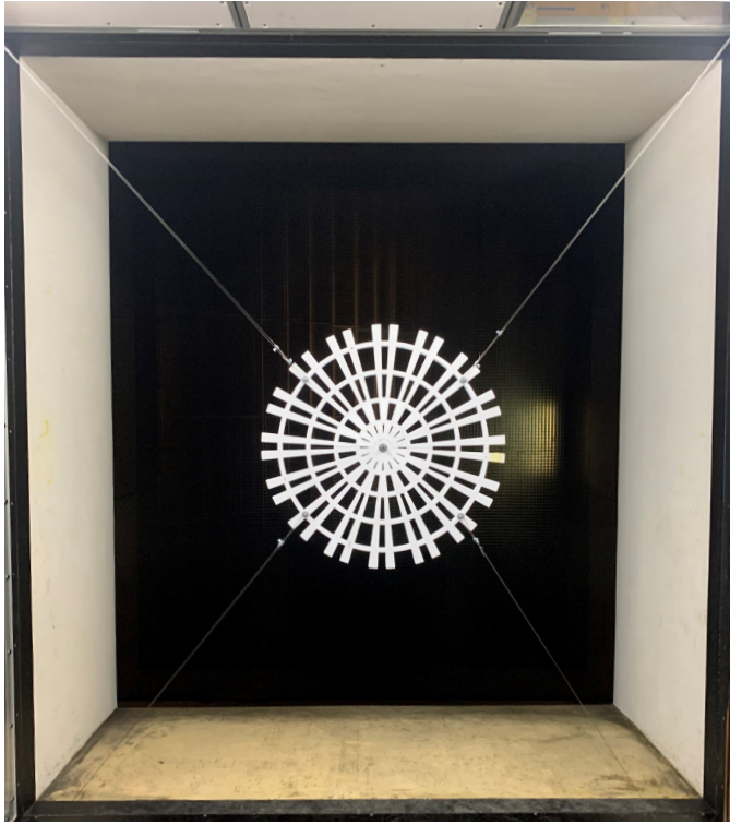
Figure 3. Porous disk (left) and porous cylinder (right) installed at the inlet of the test section, as used in part of this study. The diameters of the disk and the cylinder are of 0.5 m and 0.25 m, respectively.
