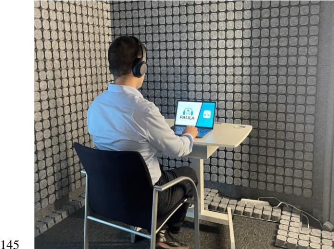
145 Figure 2: Laboratory setup used for the listening experiment (source: authors' own).
