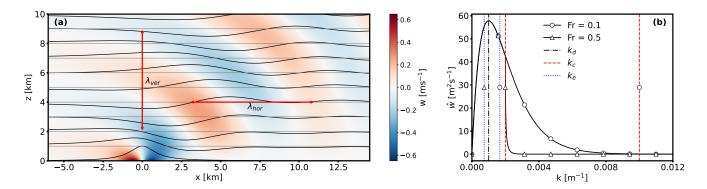
Figure 2. (a) Steady-state analytical solution of flow over a WOA hill centered at x = 0km. The color contours represent vertical velocity, and the streamlines from the displacement field show the wave propagation of the waves. (b) The streamwise wave spectrum for vertical velocity at a height, where critical, dominant, and effective wavenumbers are identified for  $F_T = 0.1$  and 0.5. Allaerts (2022)
