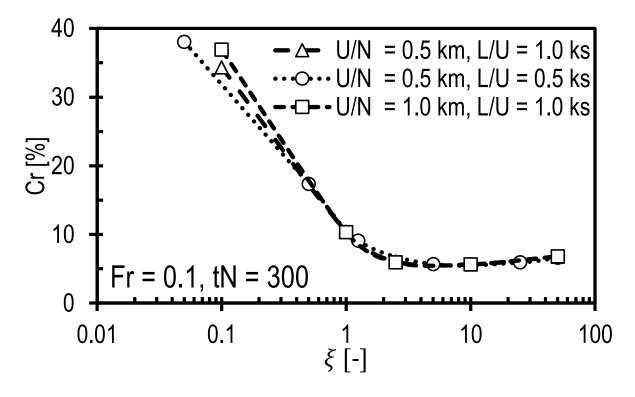
Figure 6. Reflection coefficient as a function of normalised damping coefficient  $\xi$  for varying length and time scales.
