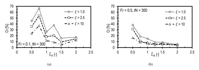
Figure 9. Reflection coefficient for the hill case as a function of normalised damping layer thickness for different values of the damping coefficient when (a) Fr = 0.1 and (b) Fr = 0.5.
