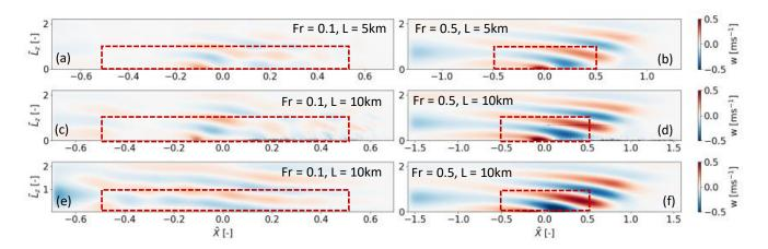
Figure 12. Plots (a-d) show vertical velocity of flow through and around the wind farm canopy with lengths L = 5 and 10 km for Fr = 0.1 and 0.5, and  $\tilde{X} = 1.0$ . For comparison, the plots (e-f) show the corresponding hill cases where L = 10 km for Fr = 0.1 and 0.5, and  $\tilde{X} = 1.0$ . The region inside the dashed red box is the non-damped domain.
