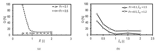
Figure 13. Reflection coefficient for the wind farm canopy case as a function of: (a) domain length for Fr = 0.1 and Fr = 0.5 for L = 5 km and  $\frac{10 \text{ km}; \text{ and }}{10 \text{ km}; \text{ and }}$  (b) domain height for Fr = 0.1,  $\tilde{L}_d = 1.5$  and Fr = 0.5,  $\tilde{L}_d = 1.2$ .
