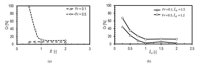
Figure 13. Reflection coefficient for the wind farm canopy case as a function of: (a) domain length for Fr=0.1 and Fr=0.5 for L=5 km, and  $\frac{10 \text{ km}}{3}$ ; and  $\frac{10 \text{ km}}{3$
