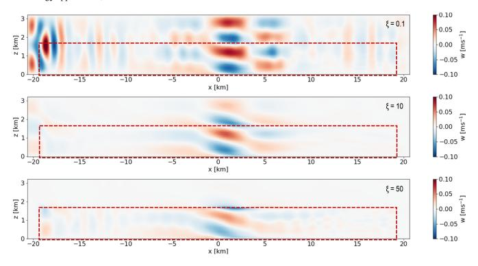
Figure 7. Contours of vertical velocity in a streamwise-oriented vertical plane at tN 300 for Fr=0.1 with  $\xi=0.1$  (top),  $\xi=10$  (middle), and  $\xi=50$  (bottom). The red box shows the non-damped domain, and everything outside is the RDL.
