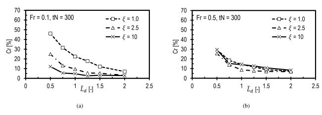
Figure 11. Reflection coefficient for the wind farm canopy case as a function of normalised damping layer thickness for different values of the damping coefficient when (a) Fr = 0.1 and (b) Fr = 0.5.
