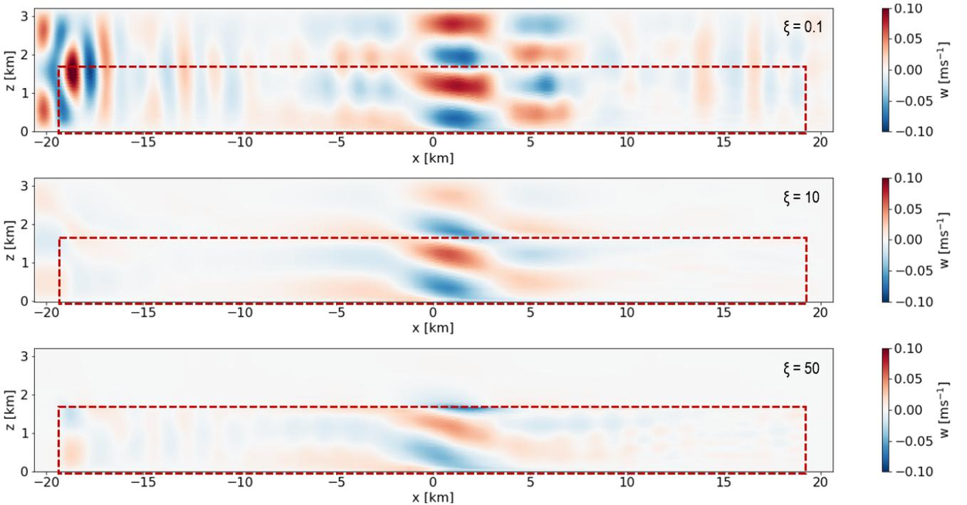
**Figure 7.** Contours of vertical velocity in a streamwise-oriented vertical plane at  $tN = 300$  for  $Fr = 0.1$  with  $\xi = 0.1$  (top),  $\xi = 10$  (middle), and  $\xi = 50$  (bottom). The red box shows the non-damped domain, and everything outside is the RDL.
