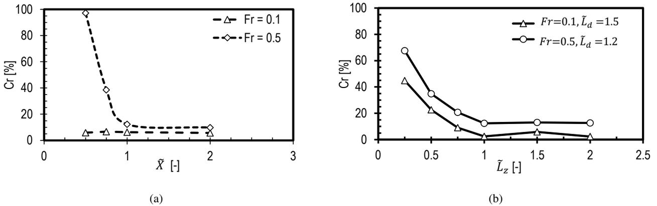
**Figure 13.** Reflection coefficient for the wind farm canopy case as a function of: (a) domain length for  $Fr = 0.1$  and  $Fr = 0.5$  for  $L = 5$  km and  $10$  km; and (b) domain height for  $Fr = 0.1$ ,  $\tilde{L}_d = 1.5$  and  $Fr = 0.5$ ,  $\tilde{L}_d = 1.2$ .
