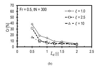
Figure 9. Reflection coefficient for the hill case as a function of normalised damping layer thickness for different values of the damping coefficient when (a) Fr = 0.1 and (b) Fr = 0.5.
