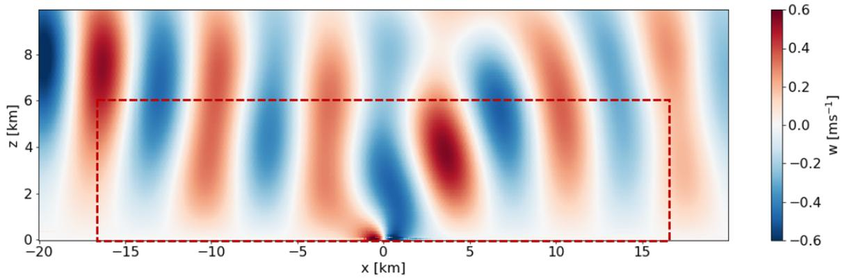
**Figure 1.** Vertical velocity contours of the flow over a small hill located at  $x = 0$  km, produced by simulating a bell-shaped hill under linearly stratified laminar conditions in SOWFA. The region outside the red dotted box consists of Rayleigh damping layers at the inlet (left), top, and outlet (right).
