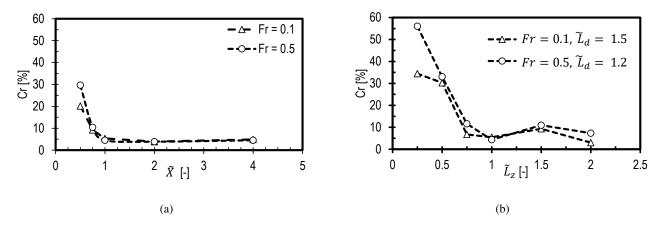
Figure 10. Reflection coefficient for the hill case as a function of: (a) domain length for Fr = 0.1 and Fr = 0.5 for L = 5 km and 10 km; and (b) domain height for Fr = 0.1,  $\tilde{L}_d = 1.5$  and Fr = 0.5,  $\tilde{L}_d = 1.2$ .
