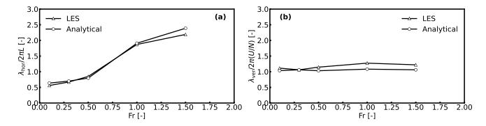
**Figure 3.** The variation of effective (a) Effective horizontal wavelength as a function of Fr, and (b) effective, dominant and buoyancy vertical wavelengths identified for Fr = 0.1 and 0.5 with Fr.
