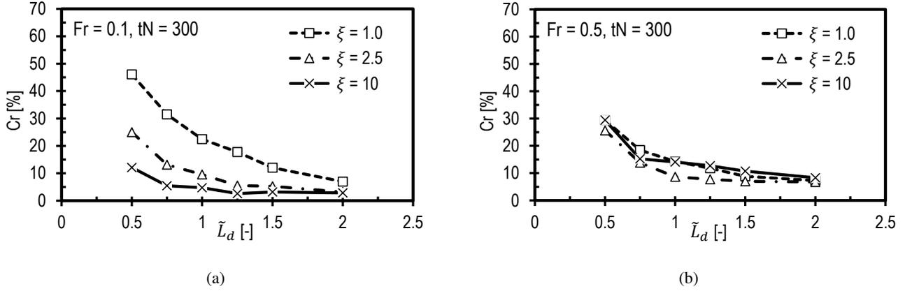
**Figure 11.** Reflection coefficient for the wind farm canopy case as a function of normalised damping layer thickness for different values of the damping coefficient when (a)  $Fr = 0.1$  and (b)  $Fr = 0.5$ .
