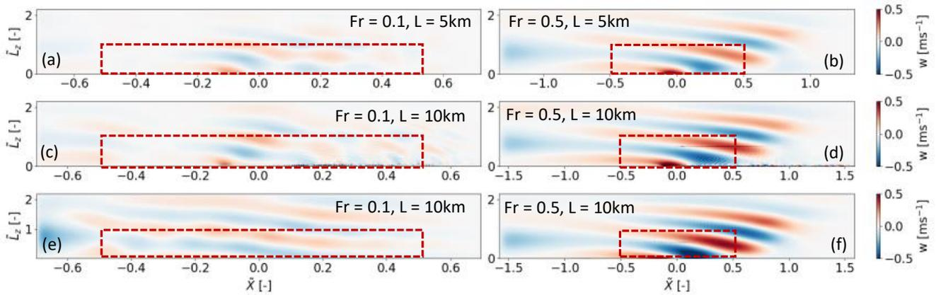
**Figure 12.** Plots (a-d) show vertical velocity of flow through and around the wind farm canopy with lengths  $L = 5$  and  $10$  km for  $Fr = 0.1$  and  $0.5$ , and  $\tilde{X} = 1.0$ . For comparison, the plots (e-f) show the corresponding hill cases where  $L = 10$  km for  $Fr = 0.1$  and  $0.5$ , and  $\tilde{X} = 1.0$ . The region inside the dashed red box is the non-damped domain.
