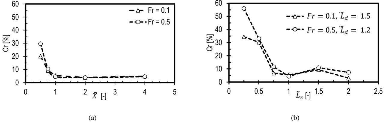
**Figure 10.** Reflection coefficient for the hill case as a function of: (a) domain length for  $Fr = 0.1$  and  $Fr = 0.5$  for  $L = 5$  km and 10 km; and (b) domain height for  $Fr = 0.1, \tilde{L}_d = 1.5$  and  $Fr = 0.5, \tilde{L}_d = 1.2$ .
