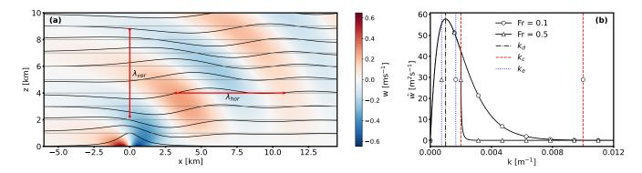
Figure 2. (a) Steady-state analytical solution of flow over a WOA hill centered at x = 0km. The color contours represent vertical velocity, and the streamlines from the displacement field show the wave propagation of the waves. (b) The streamwise wave spectrum for vertical velocity at a height, where critical, dominant, and effective wavenumbers are identified for Fr = 0.1 and 0.5. Allaerts (2022)
