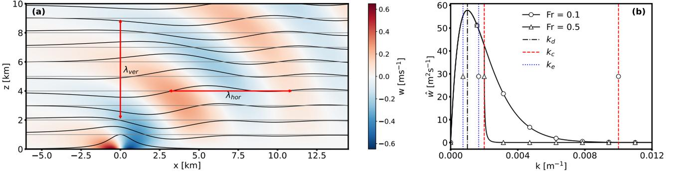
**Figure 2.** (a) Steady-state analytical solution of flow over a WOA hill centered at  $x = 0\text{ km}$ . The color contours represent vertical velocity, and the streamlines from the displacement field show the wave propagation of the waves. (b) The streamwise wave spectrum for vertical velocity at a height, where critical, dominant, and effective wavenumbers are identified for  $Fr = 0.1$  and  $0.5$ . Allaerts (2022)
