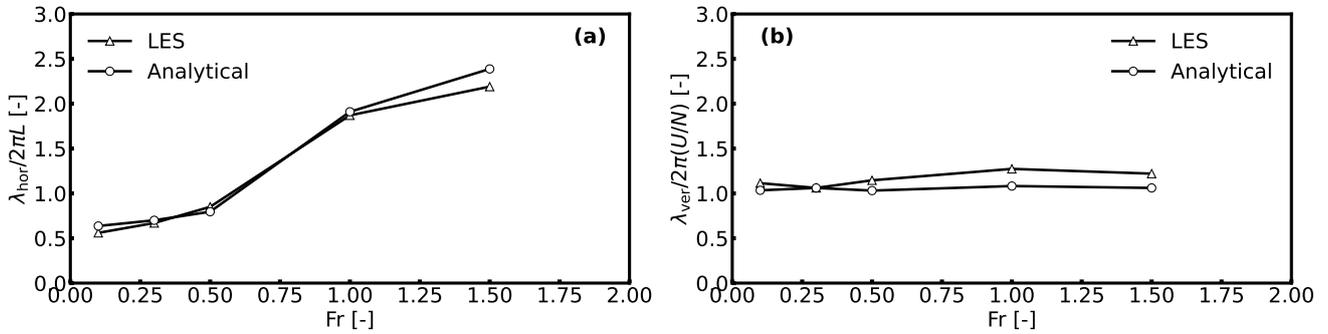
**Figure 3.** The variation of effective (a) Effective horizontal wavelength as a function of  $Fr$ , and (b) effective, dominant and buoyancy vertical wavelengths identified for  $Fr = 0.1$  and  $0.5$  with  $Fr$ .
