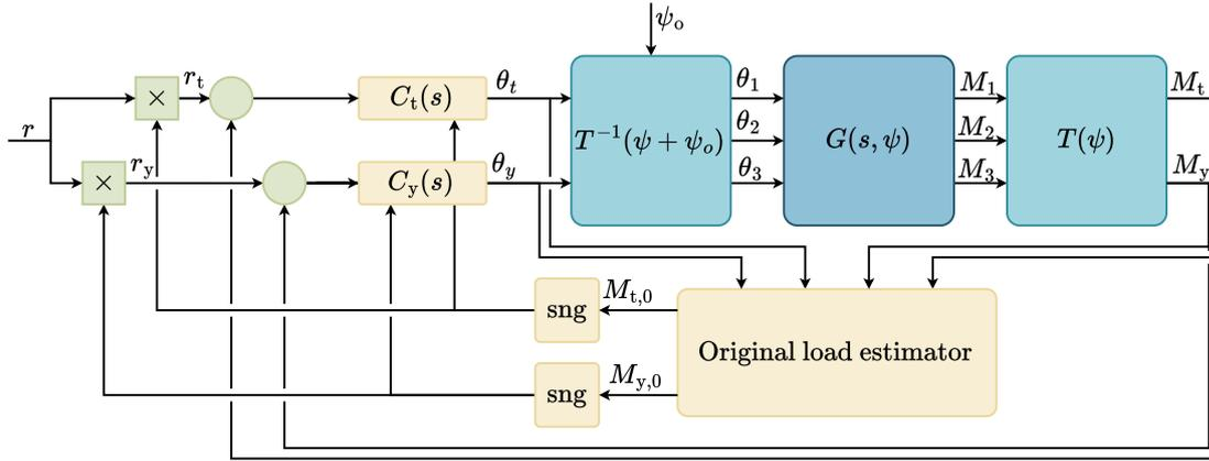
**Figure 8.** Block diagram of  $\ell^\infty$ -IPC. It uses a decoupled tilt and yaw controller that both drive the moment to the reference. To avoid load amplification, the reference sign and integrator saturation are adjusted based on the sign of the original open-loop load.
