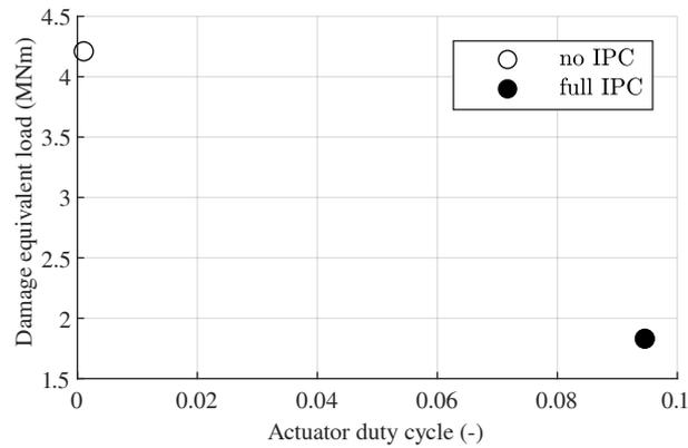
**Figure 4.** Trade-off between DEL and ADC for full IPC in laminar wind conditions. Controller tuning has no effect since the controllers reach a steady-state operating condition. So the only trade-off is to turn IPC on or off.
