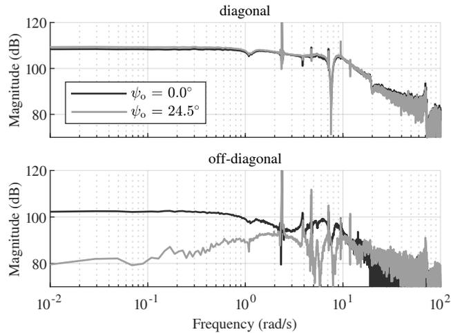
**Figure 3.** Frequency response of the demodulated plant with and without the optimal azimuth offset of  $24.5^\circ$  at a wind speed of 15 m/s. When including the azimuth offset, the off-diagonal gain is significantly reduced at low frequencies, effectively decoupling the system at those frequencies.
