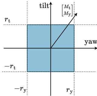
**Figure 7.** Using  $\ell^\infty$ -IPC, the nonrotating load vector is independently driven to a tilt and yaw reference  $r_t$  and  $r_y$ . The load is thus constrained within an  $\ell^\infty$ -norm, indicated by a square.
