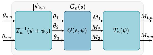
**Figure 2.** Block diagram of the demodulated plant  $\tilde{G}_n(s)$ . By calibrating the azimuth offset  $\psi_{o,n}$ , the low-frequency cross-coupling from  $\theta_t$  and  $\theta_y$  to  $M_y$  and  $M_t$  respectively, is minimized.
