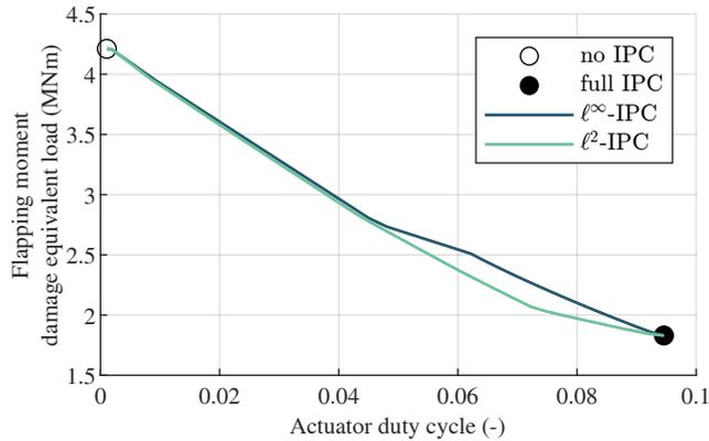
**Figure 14.** The trade-off when operating between no IPC and full IPC in laminar conditions. Especially close to full IPC,  $\ell^2$ -IPC achieves a larger reduction in the damage equivalent load of the flapping moment for the same actuator duty cycle than  $\ell^\infty$ -IPC.
