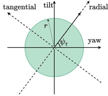
**Figure 9.** Using  $\ell^2$ -IPC, the nonrotating load vector is projected on a new orthogonal reference system, consisting of a radial and tangential axis. In this new axes system, the magnitude of the load is projected on the radial axes-axis. The load is thus constrained using the 2-norm, indicated by a circle.
