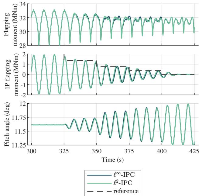
**Figure 11.** Time domain results to the staircase reference load input in the rotating frame. While both output-constrained IPC control methods follow the reference accurately, they have a slightly different control action and resulting flapping moment during the transition between no IPC to full IPC.
