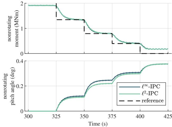
**Figure 12.** Time domain results to the staircase reference load in the nonrotating frame. Both control methods accurately follow the reference. The  $\ell^2$ -IPC controller requires a smaller nonrotating pitch magnitude, indicating that it is more efficient.
