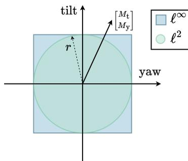
**Figure 6.** The tilt and yaw moments are visualized as a vector on the tilt-yaw plane. Output-constrained IPC then constrains this vector to a reference  $r$ . Shown here are the  $\ell^\infty$  or  $\ell^2$ -norm of the load, which form the fundament of the  $\ell^\infty$ -IPC and  $\ell^2$ -IPC control methods.
