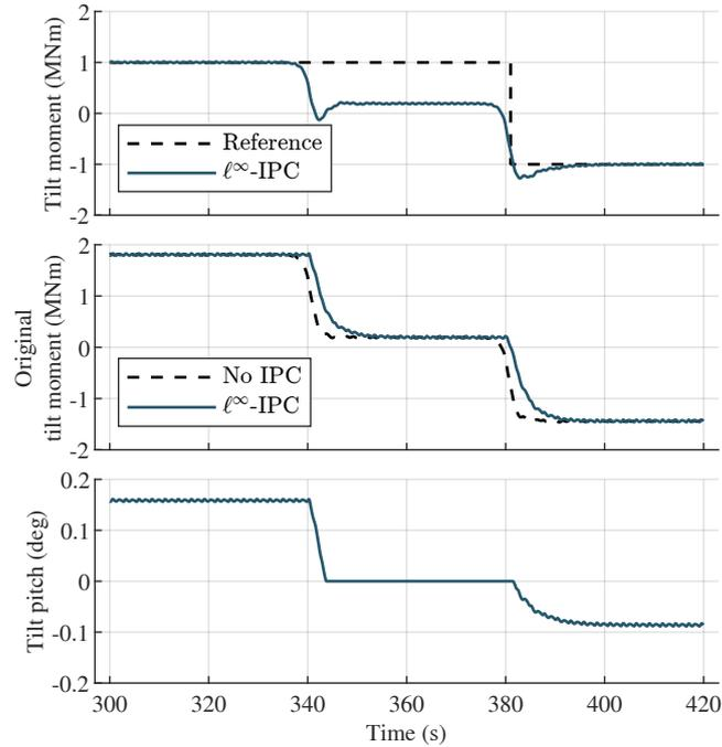
**Figure 15.** The  $\ell^\infty$ -IPC control method first follows a reference of 1 MNm accurately. At the first wind shear change, the load naturally goes below this reference and due to tilt pitch saturation, the controller does not amplify the load. Once its estimate of the [original open-loop](#) load becomes negative, just after the second wind shear change, the reference sign and the controller saturation change, allowing the controller to reduce the tilt moment to -1 MNm.
