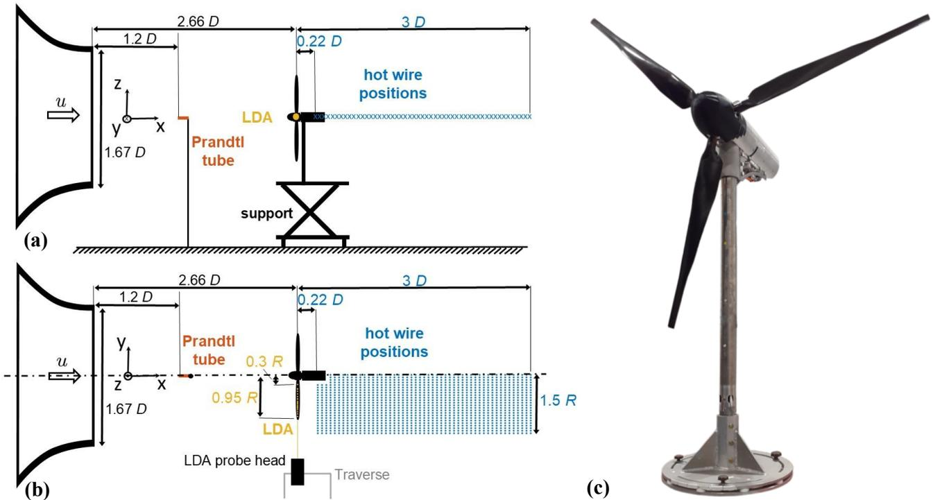
**Figure 7.** Experimental set-up, side (a) and top view (b), indicating the measurement positions of the hot wires, LDA and Prandtl tube. The coordinate system is located in the rotor centre. MoWiTO 1.8 with the Hybrid-Lambda blades (c),  $D = 1.8$  m, hub height of 1.5 m.
