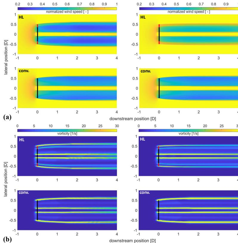
**Figure 15.** Normalized wind speed (a) in light-wind (left) and strong-wind mode (right). Vorticity magnitude (b) in light-wind (left) and strong-wind mode (right), for the Hybrid-Lambda model turbine (top) and the conventional model turbine (bottom) from FVW simulations.
