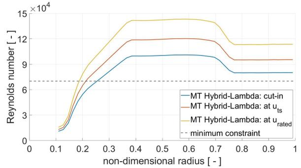
**Figure 5.** Reynolds number for three different operating modes, derived from BEM simulations
