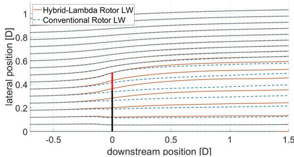
**Figure 11.** Streamlines from FVW simulations for the Hybrid-Lambda model turbine in LW mode and the conventional model turbine (same  $c_T$ ). The rotor is indicated with the vertical black bar, the low-induction tips are displayed in bright red.
