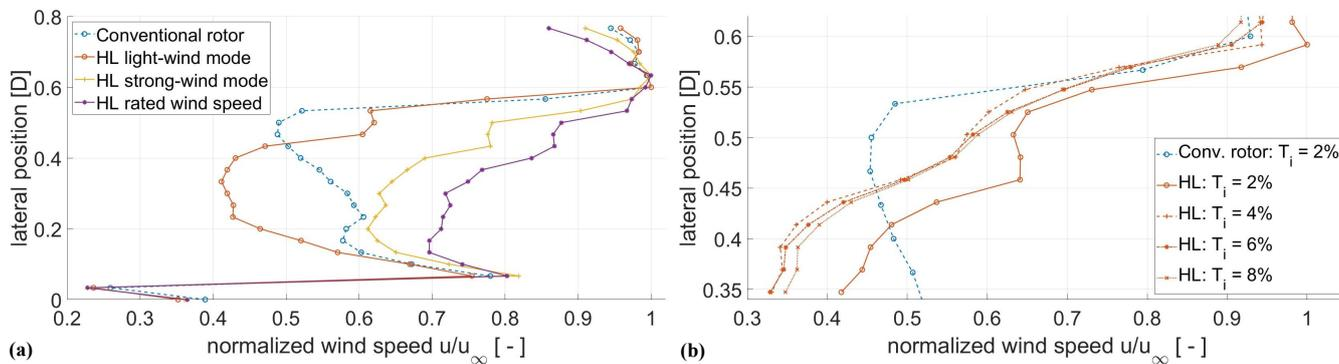
**Figure 14.** Wake profiles at  $0.4 D$  downstream distance for the two model rotors. At  $T_i = 2\%$  for different operating modes (a), in light-wind mode for different  $T_i$  (b).
