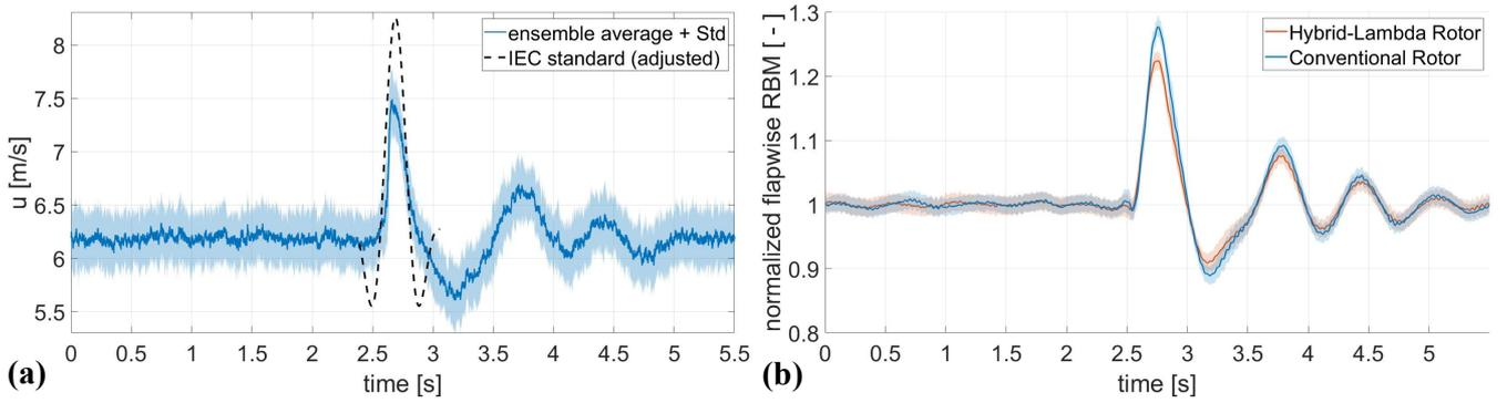
**Figure 12.** Left: Gust in the wind tunnel: Inflow hot-wire measurements in the rotor plane and scaled IEC gust, displayed 8 times slower than ideal scaling, gust amplitude is not scaled (a). Right: Flapwise RBM response of the Hybrid-Lambda and the conventional rotor. The shaded area indicates the 95% confidence interval of the 45 repetitions of the gust event (b).
