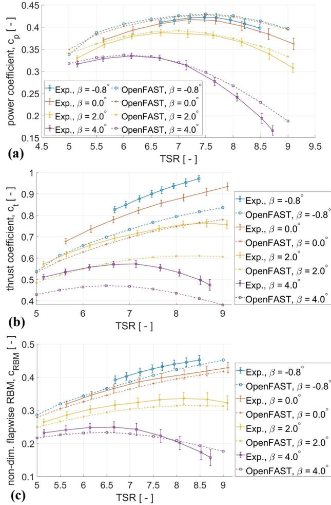
**Figure 8.** Power coefficient (a), thrust coefficient (b) and non-dimensional flapwise RBM (c) from measurements and BEM simulations for various TSR and pitch angles  $\beta_{pitch}$ , at constant rotor speed of 500 rpm.
