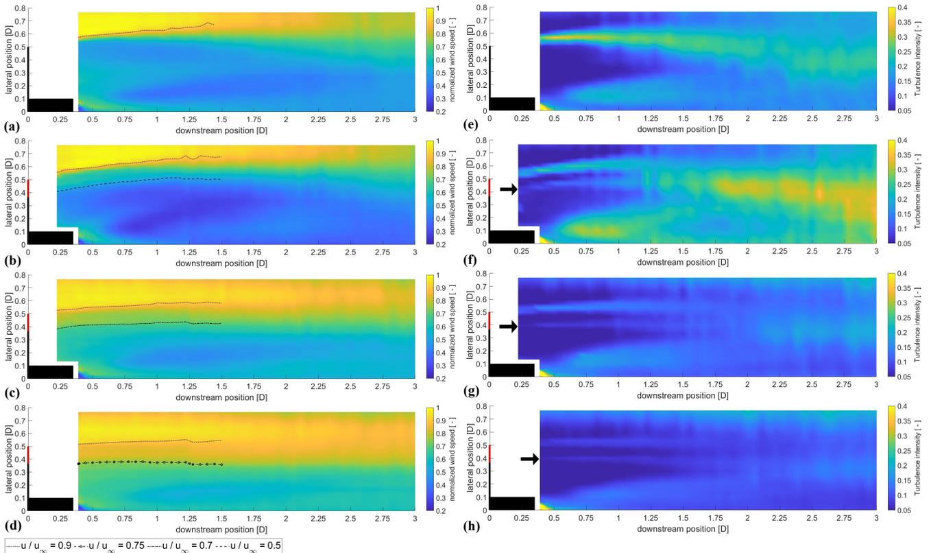
**Figure 13.** Mean normalized wind speed (a-d) and turbulence intensity (e-h) from hot-wire measurements in the wake of the model turbines. From top to bottom: Conventional rotor (a,e), Hybrid-Lambda Rotor in LW mode (b,f), SW mode (c,g) and at rated wind speed (d,h). Nacelle and blades are displayed in black, the outer 30% of the Hybrid-Lambda blades are displayed in red. The black arrows point at the second shear layer starting at the blade design blending region.
