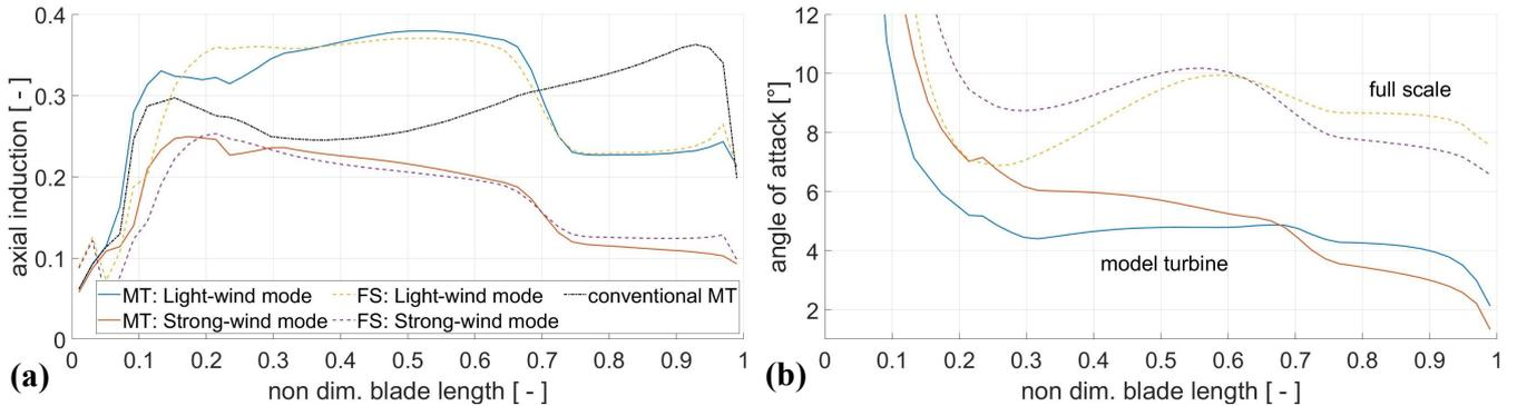
**Figure 6.** Axial induction (a) for light-wind mode (at  $u_{1s}$ ) and strong-wind mode (at  $u_{1e}$ ) for the Hybrid-Lambda model turbine (MT), the full-scale rotor (FS) and the conventional model turbine in BEM simulations and respective angle of attack distributions (b).
