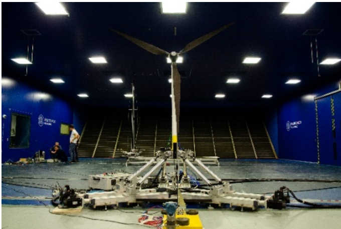
Figure 1: Experimental testcase and geometric properties of the scaled DTU 10 MW model.
