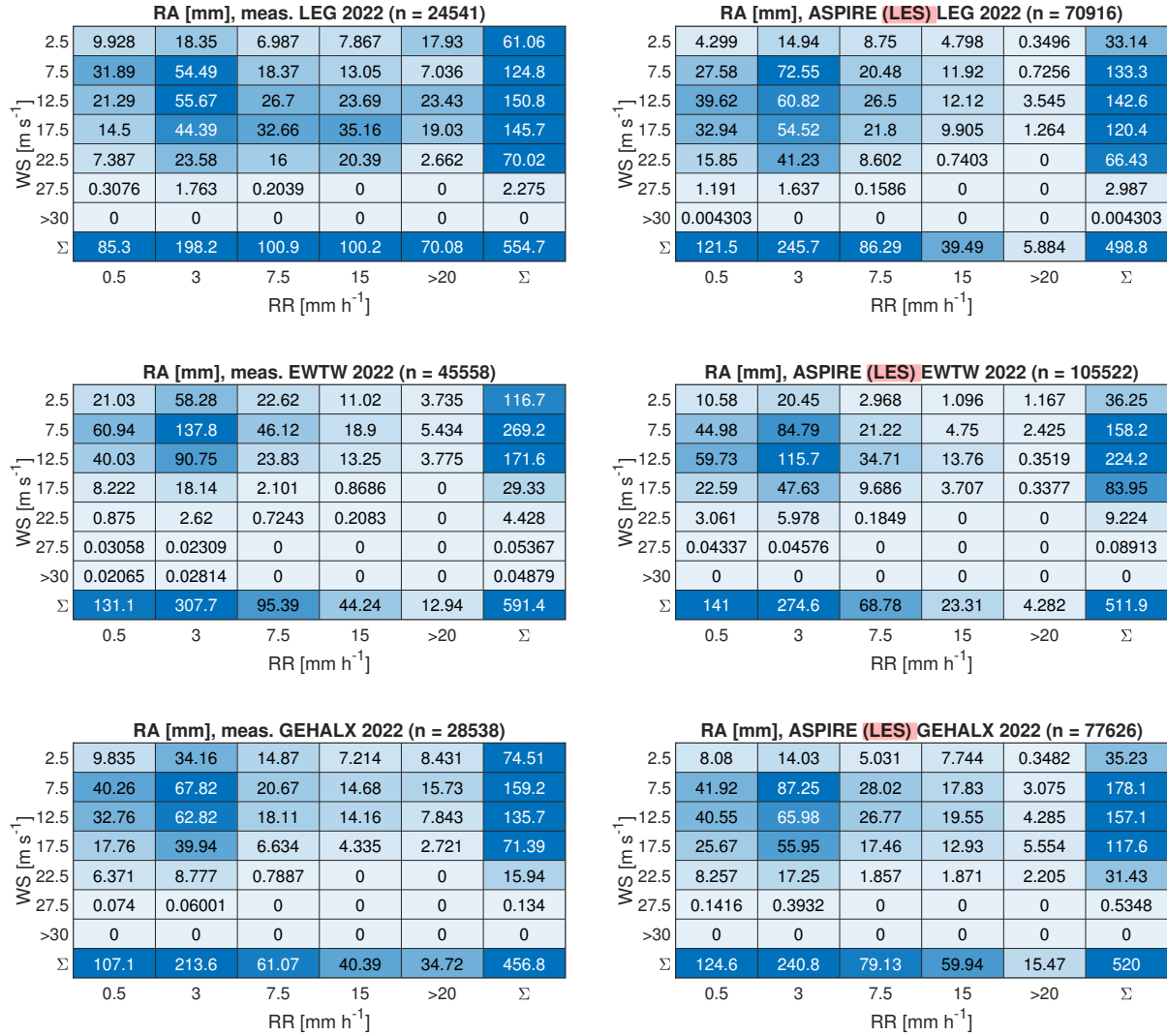
Figure 14. Annual rainfall categorized into bins based on wind speed and rain rate. Presented here are the numerical results from the high resolution LES.
