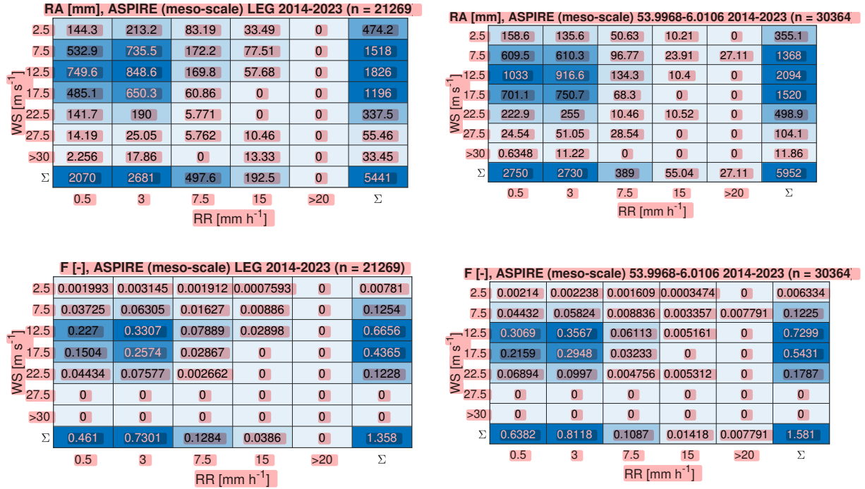
Figure 6. Yearly rain amount and accumulated damage sorted out into wind speed and rain rate bins. This figure compares a location situated in the southern part of the Dutch North Sea (LEG platform) with a location in the northeast (with coordinates 53.9968, 6.0106). The ASPIRE results presented in this figure are obtained from the meso-scale simulations.
