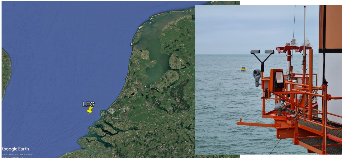
Figure 1. A map showing the location of the Lichteiland Goeree (LEG) platform, where concurrent rain and wind speed measurements were conducted (Caboni et al., 2024), and a picture of the OTT Parsivel 2 disdrometer installed on the platform. Map courtesy of © Google Earth.
