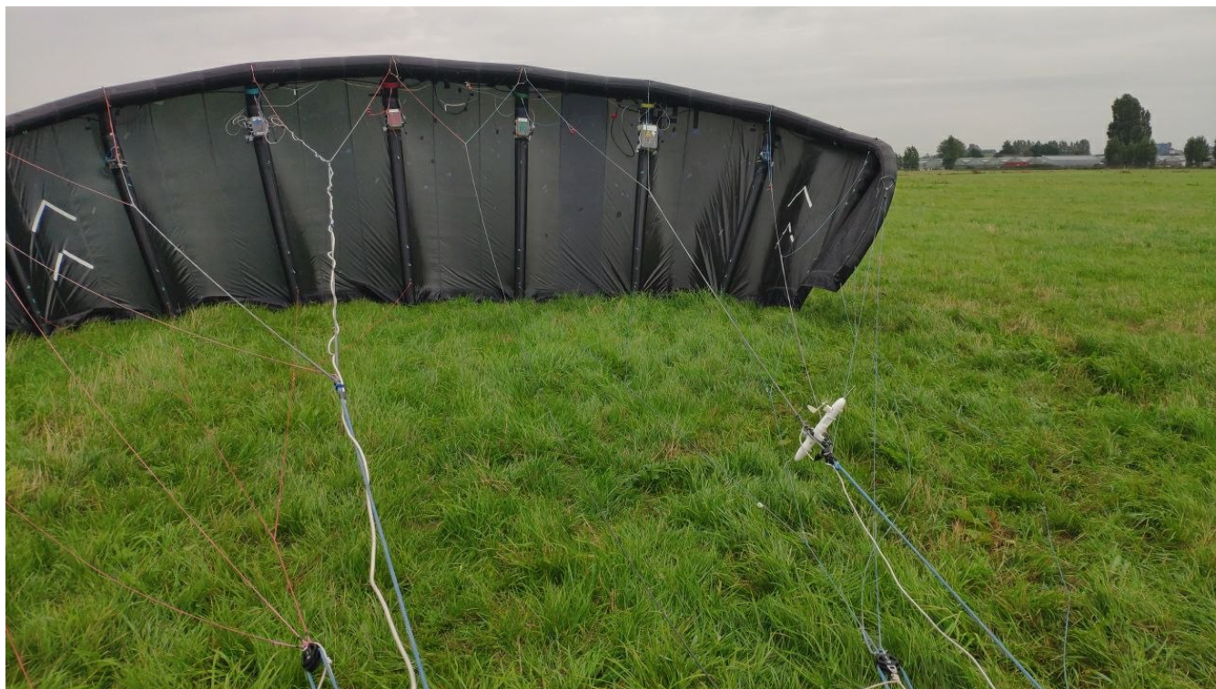
Figure 3. Fully instrumented V3.25 kite before launch. Photo courtesy of Kitepower B.V.
