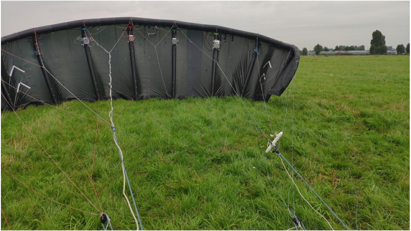
Figure 3. Fully instrumented V3.25 kite before launch. GPS+IMU units are visibly mounted in four of the inflatable struts. A Pitot tube and a wind vane are also installed in the bridle lines. Photo courtesy of Kitepower B.V.
