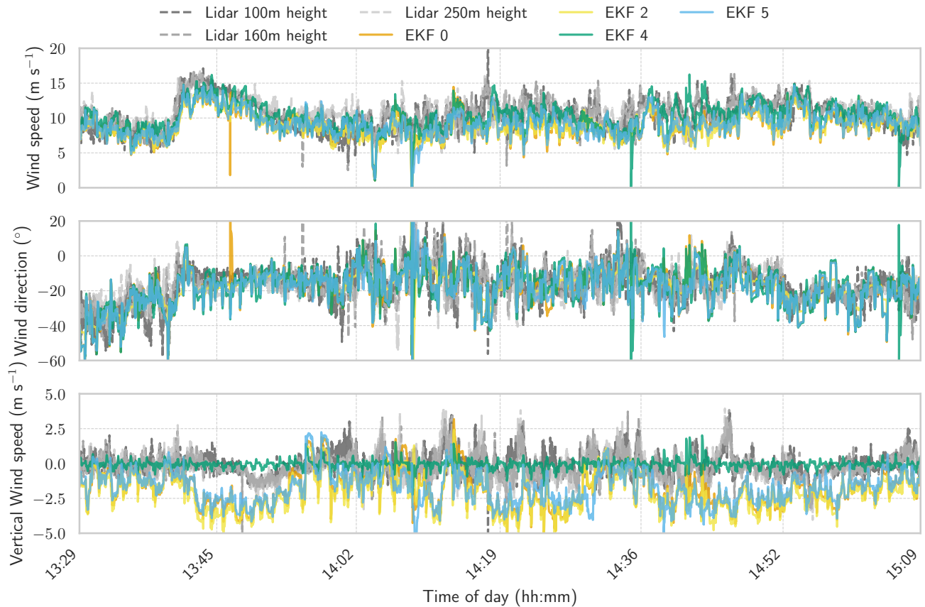
Figure 21. Test flight from 05-06-2024. Wind profile comparison between EKF results with a minimum sensor setup and lidar observations.
