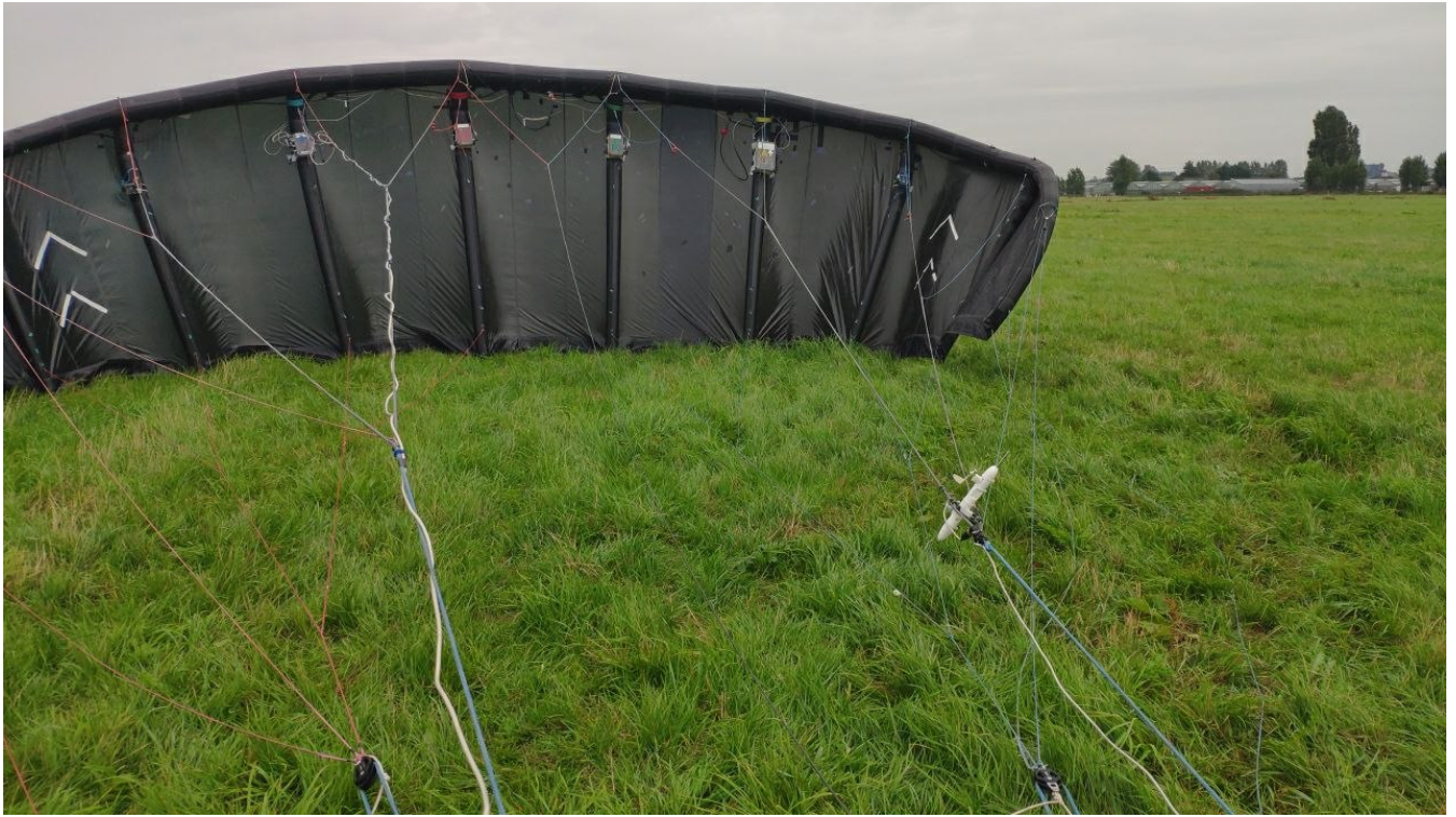
Figure 3. Fully instrumented V3.25 kite before launch. GPS+IMU units are visibly mounted in four of the inflatable struts. A Pitot tube and a wind vane are also installed in the bridle lines. Photo courtesy of Kitepower B.V.
