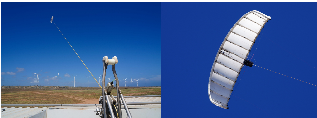
Figure 2. The V9 kite in flight: view from the ground station (left), and close-up showing the suspended control unit (right). Photos courtesy of Kitepower B.V.
