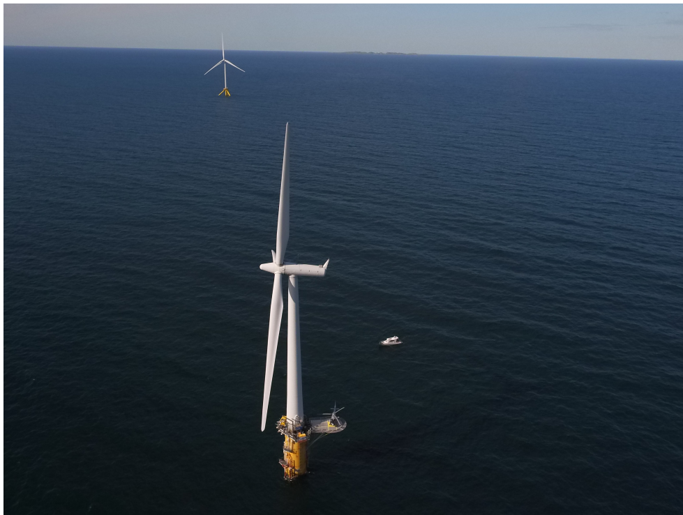
Figure 4. The Zefyros floating offshore wind turbine relies on a Siemens 2.3-MW. Credits: Unitech Energy Group
