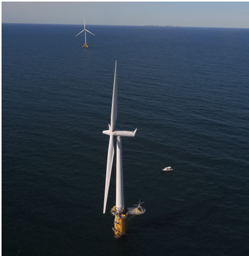
Figure 5. The Zefyros floating offshore wind turbine relies on a Siemens 2.3-MW. Credits: Unitech Energy Group
