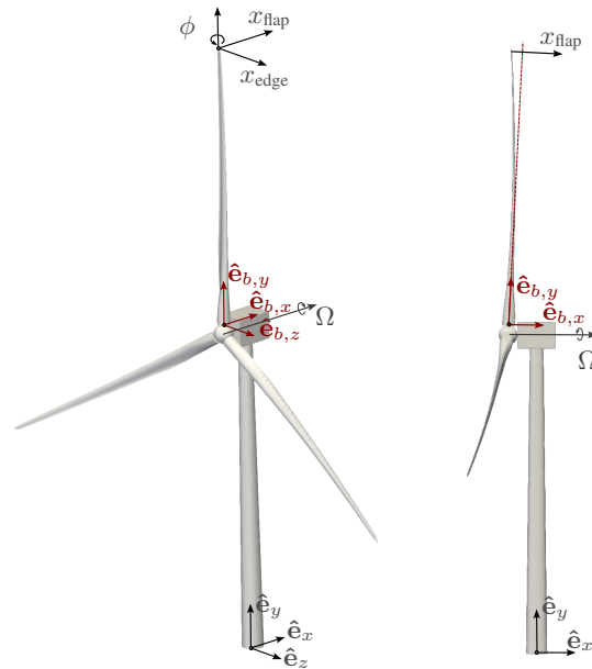
Figure 3. References frames: global frame (black, \hat{e} ) and blade root frame (red, \hat{e}_b ). The rotor rotation vector \Omega and the blade tip displacements ( x_{\text{flap}} , x_{\text{edge}} and \phi ) are also shown. 3D turbine rendering from OpenFAST.
