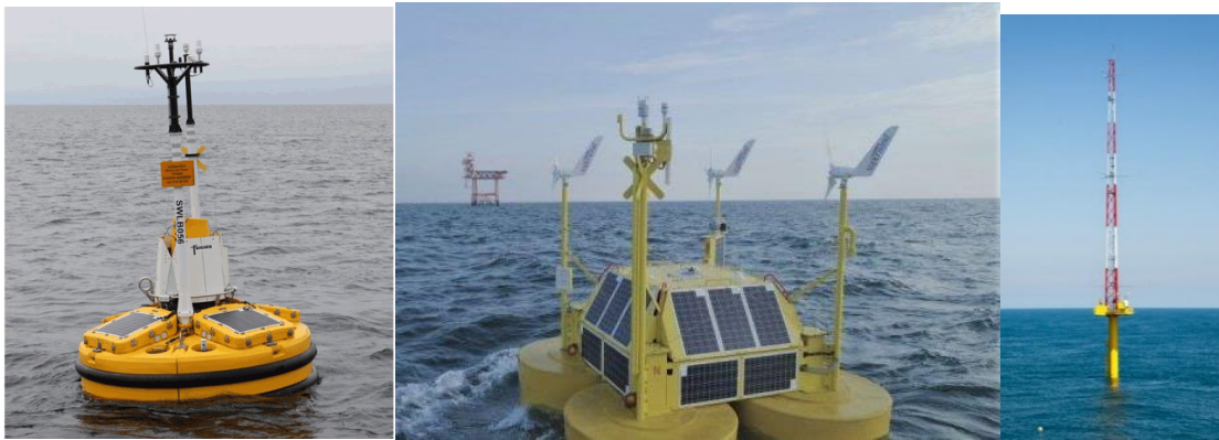
100 Figure 1: Photographs of the Floating LiDAR Systems (left: Fugro, middle: Eolos) as well as the IJmuiden mast (right). Sources: Fugro, Eolos, Wind op Zee.
