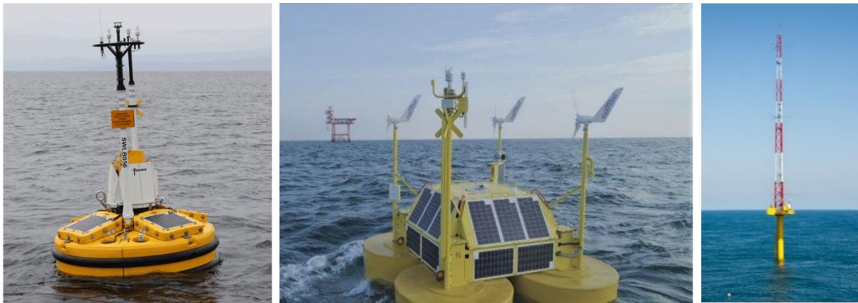
95 Figure 1: Photographs of the Floating LiDAR Systems (left: Fugro, middle: Eolos) as well as the IJmuiden mast (right). Sources: Fugro, Eolos, Wind op Zee.
