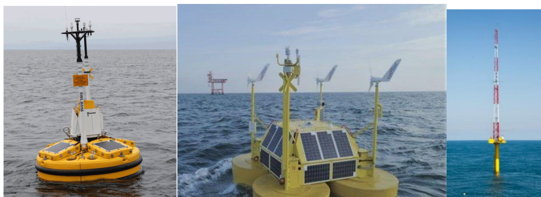
2 Figure 1: Photographs of the Floating LiDAR Systems (left: Fugro, middle: Eolos) as well as the IJmuiden mast (right). Sources: Fugro, Eolos, Wind op Zee.
