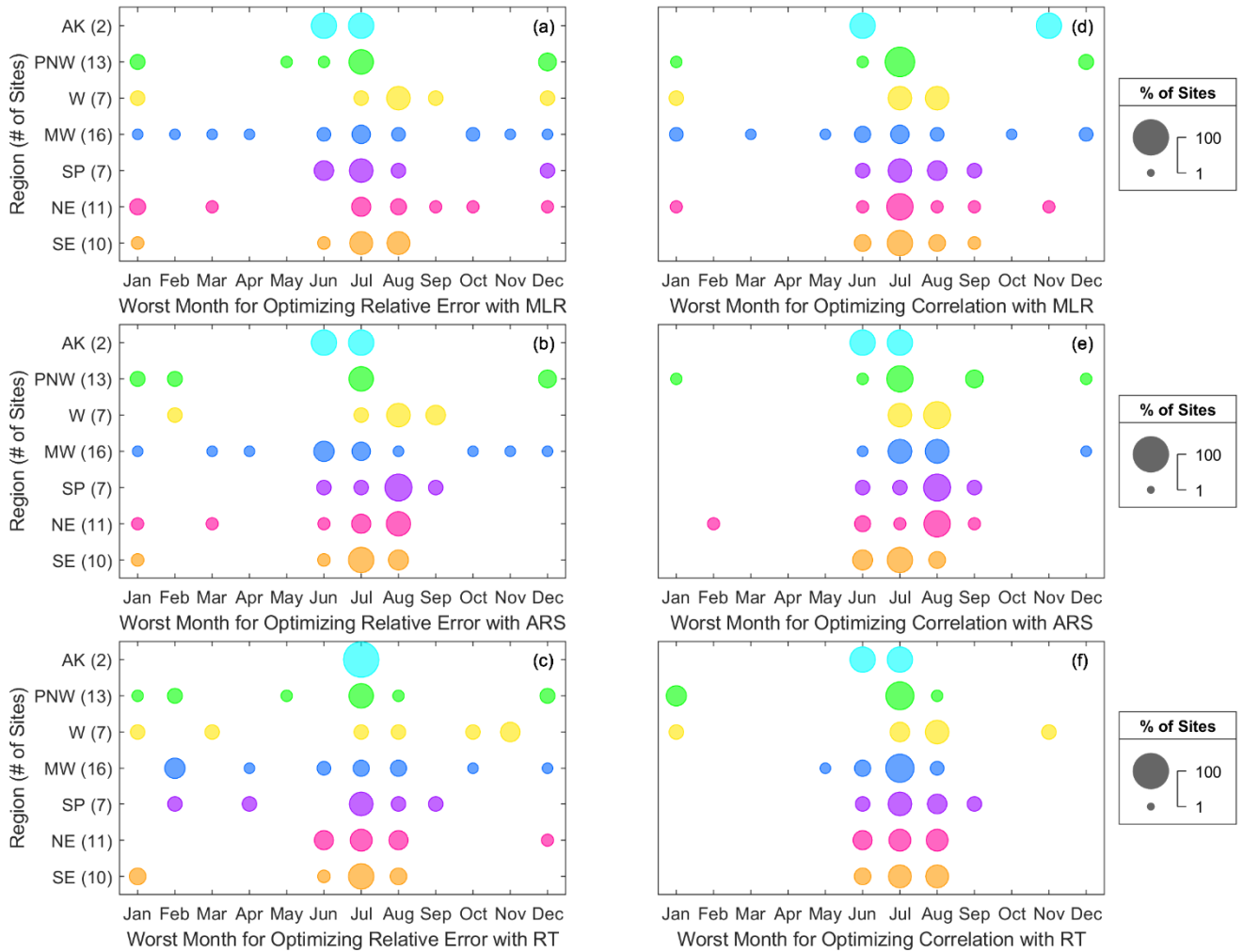
Figure 11. Worst average single months for optimizing (a), (b), (c) relative error and (d), (e), (f) correlation when creating MCP-based long-term wind speed estimates using (a), (d) MLR, (b), (e) ARS, and (c), (f) RT according to US region. Larger circles indicate the best month for more sites in a given region.
