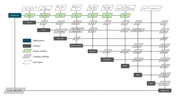
Figure 1. XDSM of the wind-farm level MDAO framework
