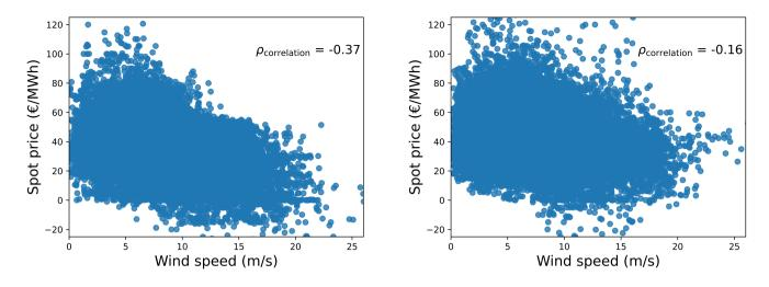
Figure 3. Correlation between spot prices and site-specific wind speeds for Denmark (left) and the Netherlands (right)
