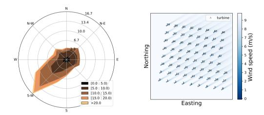
**Figure 7.** (a) Directional wind speeds and probabilities for the hypothetical site (b) Farm layout for a 15 MW turbine (and 1 GW of farm power)
