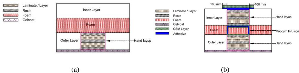
17 **Figure 17: Shear web damage - (a) Outer laminate damage, (b) Foam or inner laminated damage.**
