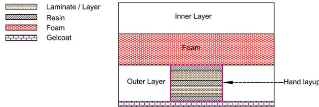
Figure 13: Outer laminate damage.
