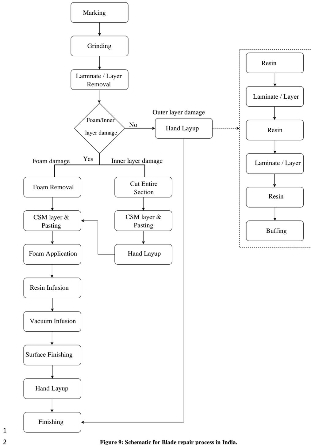
Figure 9: Schematic for Blade repair process in India.
