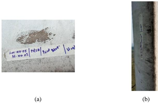
10 **Figure 11: (a) Blade eroded at an arbitrary area, (b) Leading edge eroded blade.**
