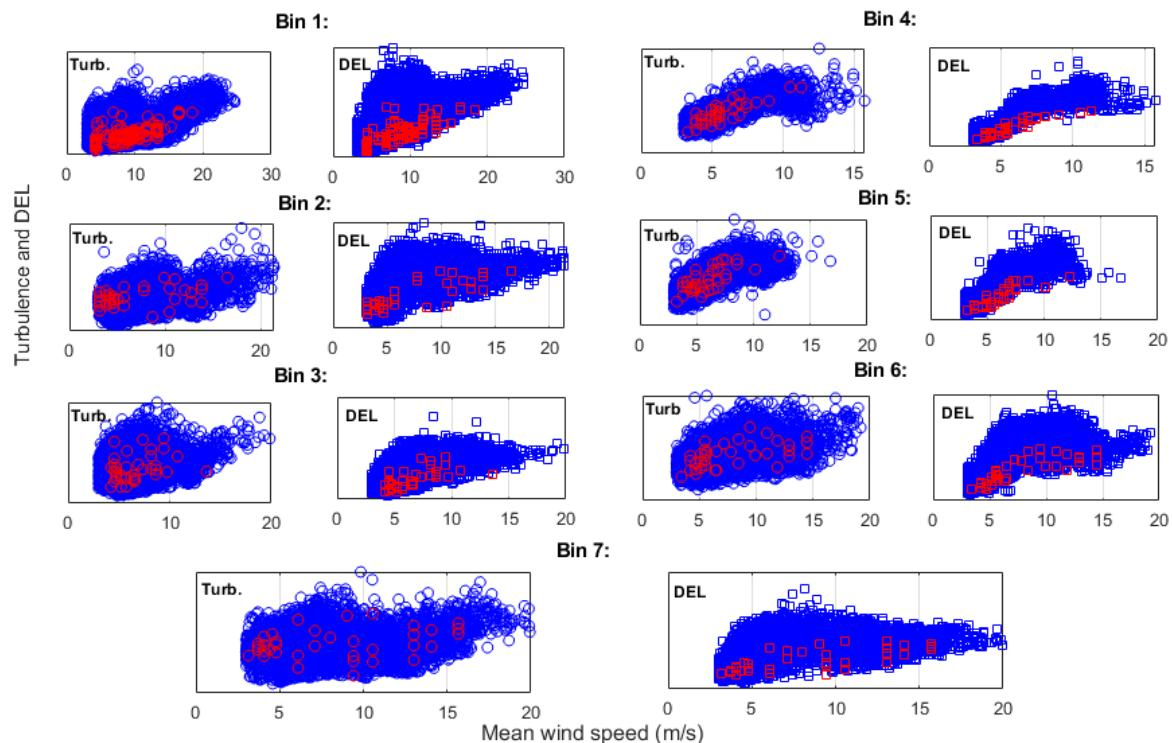
For this purpose, we took limited samples after fitting Gaussian mixture models<sup>2</sup> to wind speed and turbulence (joint distribution) and running simulations using samples covering the probability space. Below are the results in all different direction bins:
