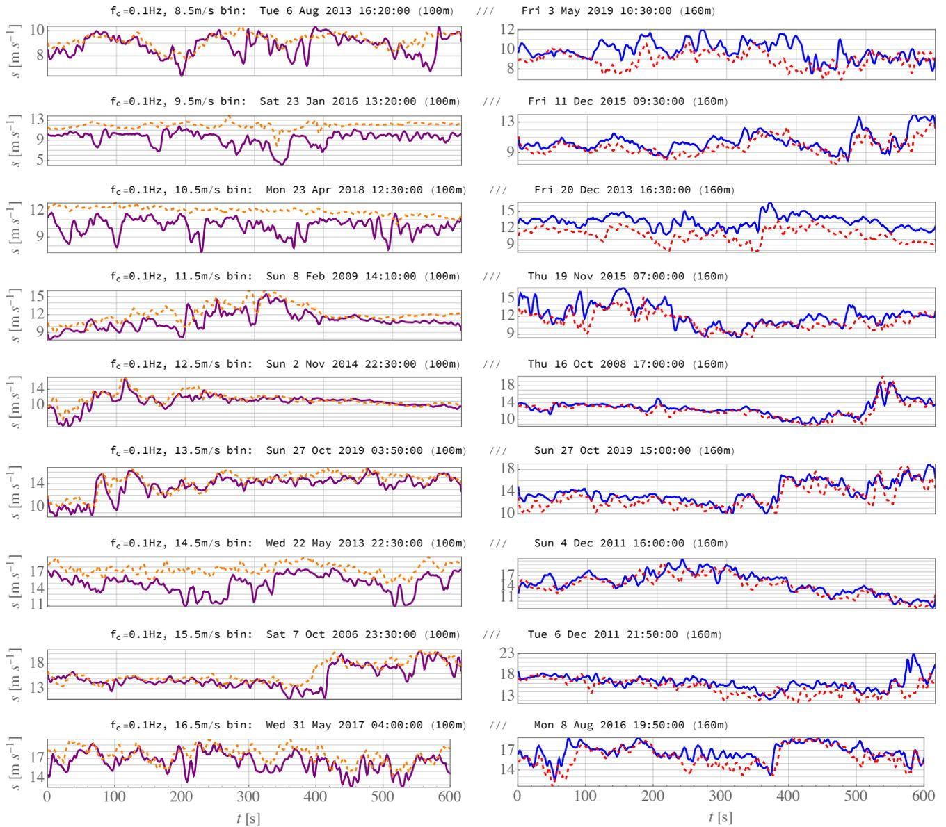
**Figure 14: pairs of 10-minute timeseries  $s(t)$ , for the most extreme acceleration events in each  $1 \text{ m s}^{-1}$  wind speed bin for low-pass filter scale of  $0.1 \text{ Hz}$ . Left: 100m events (purple  $s_e=s|_{100m}$ , dashed-orange  $s_e=s|_{100m}$ ); right: 160 m events (blue  $s_e=s|_{160m}$ , green  $s_e=s|_{100m}$ ).**
