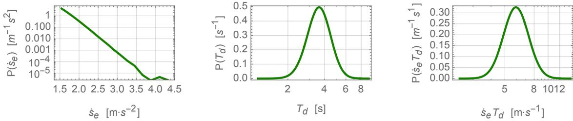
870 **Figure 18: example distributions of extreme acceleration (left), event duration (center), and associated wind speed jump (right) synthesized for simulation;  $P(\dot{s}_e)$  used corresponds to  $f_c = 1/3 \text{ Hz}$  at height of 100 m.**
