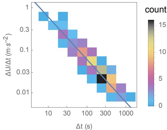
850 **Figure 17: joint PDF of bulk accelerations and rise times from the ramp data of Kelly *et al.* (2021). Solid line is  $(6 \text{ m s}^{-1})/\Delta t$ .**
