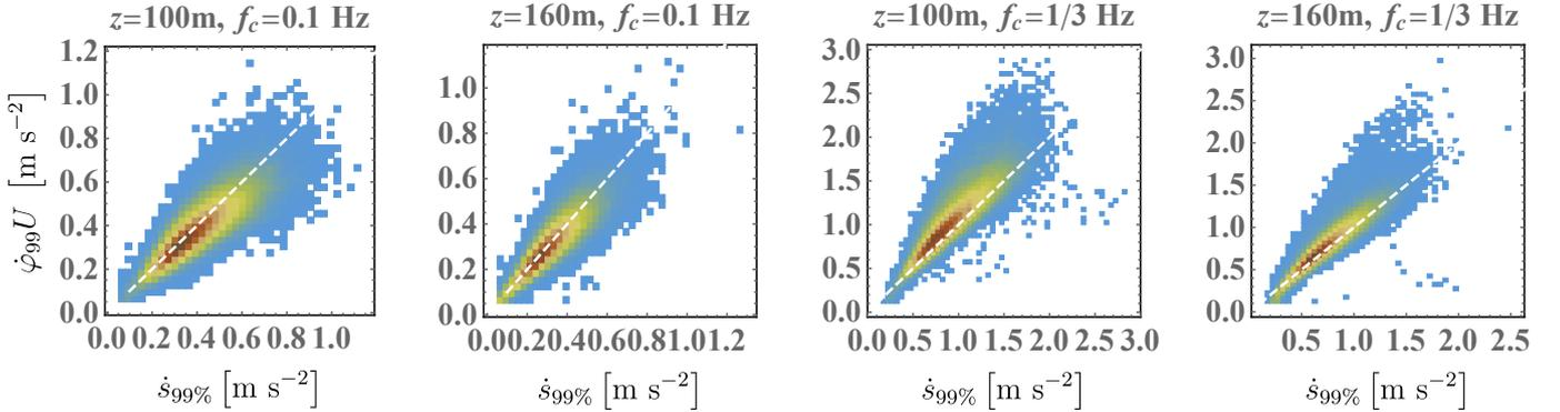
490 **Figure 12: joint PDF of 99<sup>th</sup> percentile of directional and horizontal flow accelerations, calculated as  $\dot{\phi}U$  and  $\dot{s}$ , respectively; plotted at both 100 m and 160 m heights, for characteristic response times ( $f_c^{-1}$ ) of 10 s (left) and 3 s (right). Note linear axes are used here; log-log plots give jPDF shapes similar to those shown in Figs. 6,7, and 9. Dashed white line indicates 1:1 relation.**
