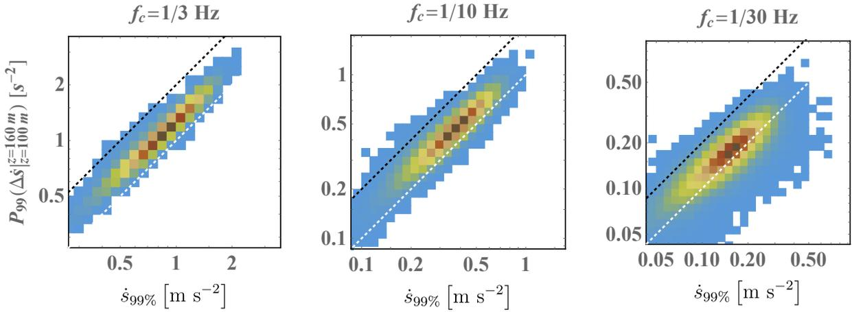
400 **Figure 9:**  $P_{99}$  of difference in low-pass filtered accelerations between 100 m and 160 m, versus  $P_{99}$  of low-pass filtered accelerations averaged over the two heights (plotted joint PDF), for all three low-pass filter scales considered. Dotted white line shows 1:1 relationship, dotted black is 2:1.
