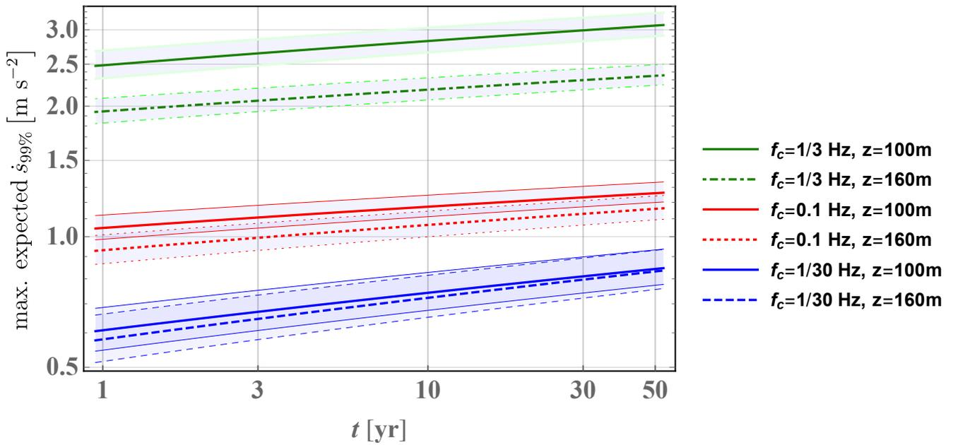
Figure 15: ~~maximum filtered acceleration expected~~: Expected  $\dot{s}_{99}$  per return period  $t$ , for the three different filter scales considered and two heights analyzed. For each case, thick lines correspond to  $T_{\text{base}} \approx 39$  minutes (total timespan divided by number of samples); shaded areas and thin lines around each case show range for base-periods varying from 10–119 minutes (see text for explanation).
