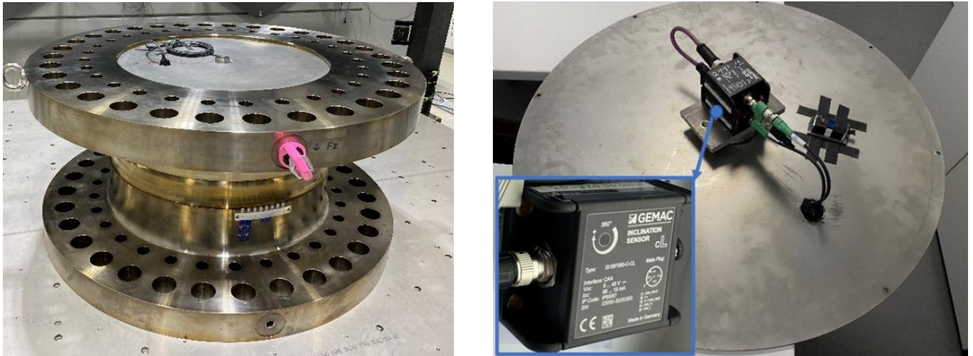
Figure 2. The 5 MN·m TTS manufactured by HBM (left image). It is a hollow-shaft transducer with flanges to be mounted in test benches. In the left image, the hollow-shaft is covered by a cover plate. On the inside of this cover and placed centred is the inclinometer stack (zoom in right image). Moreover, a small sensor to log temperature and humidity inside the TTS is taped to the inner side of the cover plate (right image, black tape). Taken from (Song et al., 2022).
