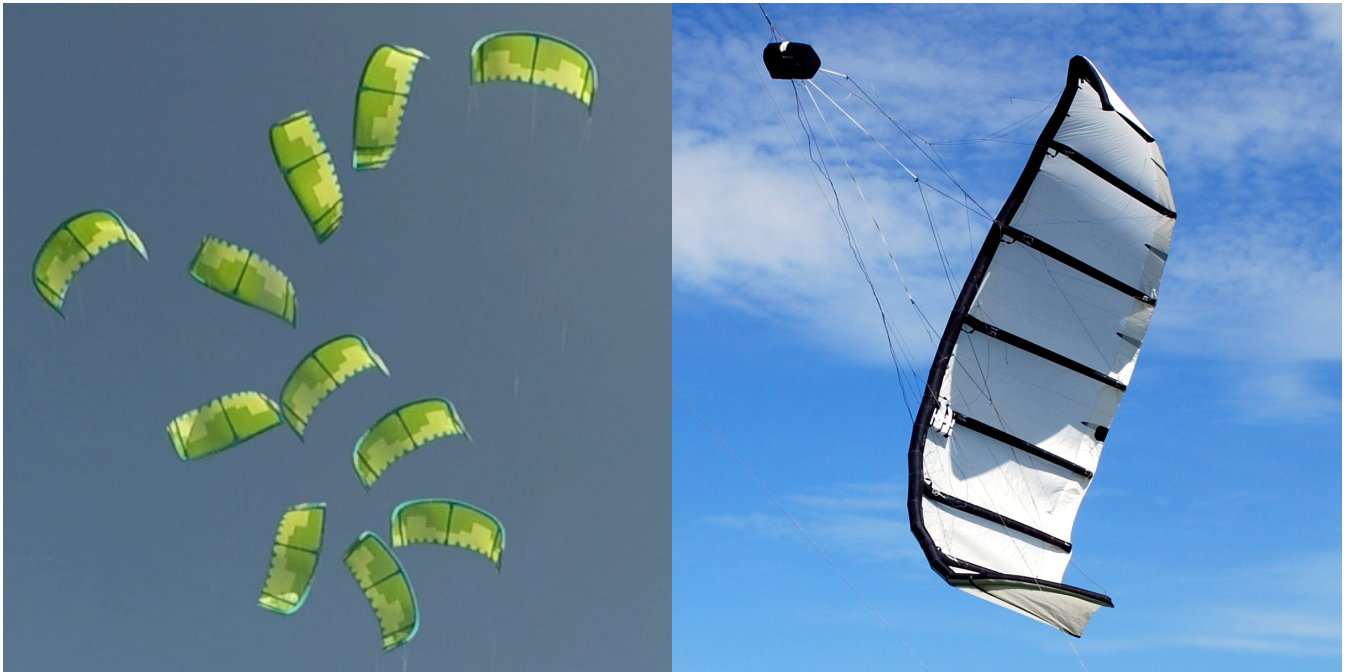
Figure 1. Time-lapse composite photo of a 6 m 2 power kite for sport applications performing a sharp turn to the left and subsequent loop manoeuvre, taken from the towing vehicle, from Lange (2018) (left). Photo of a 25 m 2 power kite for airborne wind energy applications performing turn to the right during a mast-based launch manoeuvre, reported by Oehler and Schmehl (2019) (right). Both photos illustrate the spanwise twist deformation exhibited by LEI kites. The extreme deformation in the right photo does not occur in regular flight operations but resulted from mast-based launch attempts, shown here only to visualise the wing twist mechanism.
