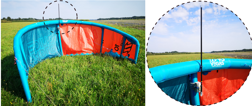
Figure 15. The Vegas 2015 kite with mounted Prandtl tube, adapted from Elfert (2021).
