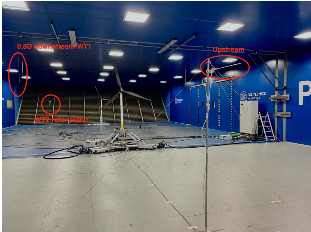
Figure 1. Locations of wind speed measurement in the wind tunnel test section.
