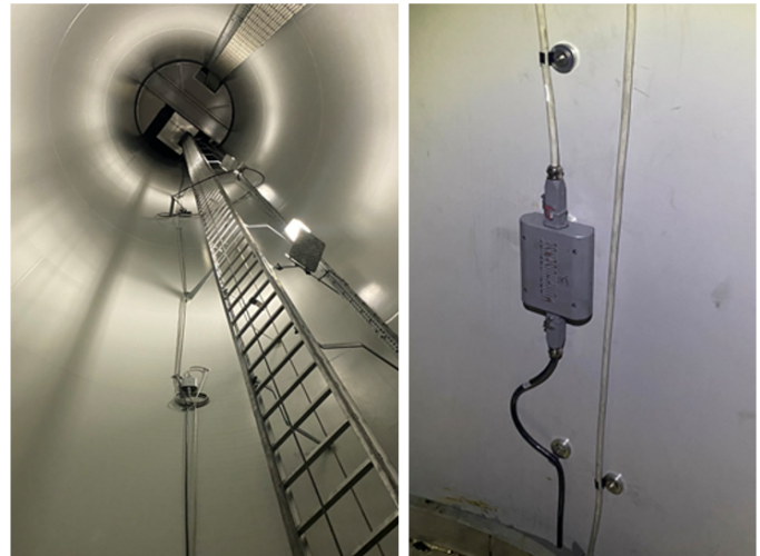
Figure 2. Zephyros, Sensor position along the world's first multi-megawatt FOWT UNITECH (2022) tower. Credits: Unitech Energy Group
