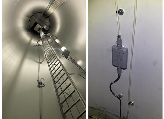
Figure 2. Sensor position along the tower.
