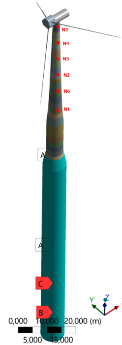
Figure 3. Graphic representation of the finite element model used in Homer software
