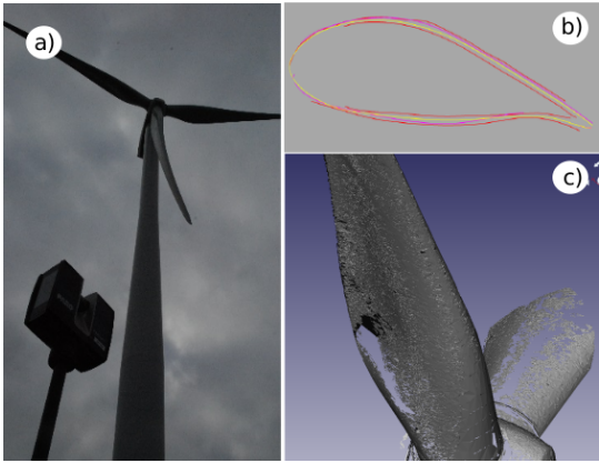
Figure 10. First blade scan operation: (a) 3D scanner on the ground close to the wind turbine, (b) scatter of possible blade sections that can be extracted from the cloud of points, (c) missing data (“holes”) in the measured cloud of points from this first scan operation.
