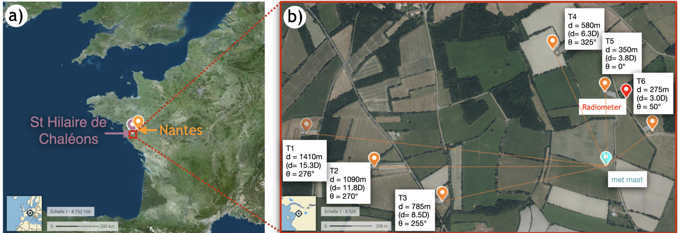
Figure 1. Overview of the measurement site (b) at Saint-Hilaire-de-Chaléons in the west of France (a). The site is 10 km from the coast and 32 km from Nantes. The site consists of six wind turbines with different distances d from the met mast (b). Aerial photo source: ©IGN – « BD ORTHO® ».
