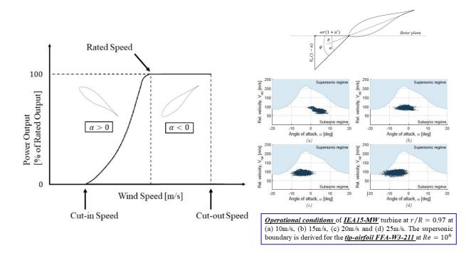
Figure 1: Sketch of a power curve (left), sketch of the angle of attack distribution for wind turbine airfoil (right-up), and operational conditions for IEA-15MW RWT tip airfoil from De Tavernier and von Terzi, 2022 (right-down)
