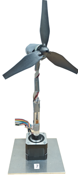
Figure 5. Photo of one of the turbine assemblies, displaying the rotor, the generator behind it, the tower with strain gauges and the stepper motor at the base.
