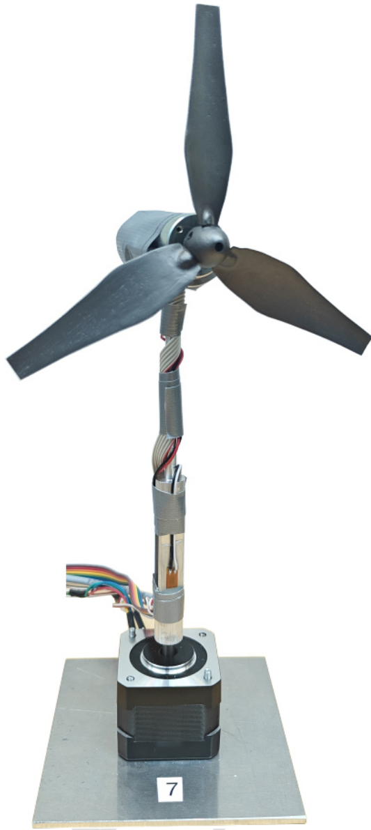
Figure 5. Photograph of one of the turbine assemblies, displaying the rotor, the generator behind it, the tower with strain gauges, and the stepper motor at the base. TS7
