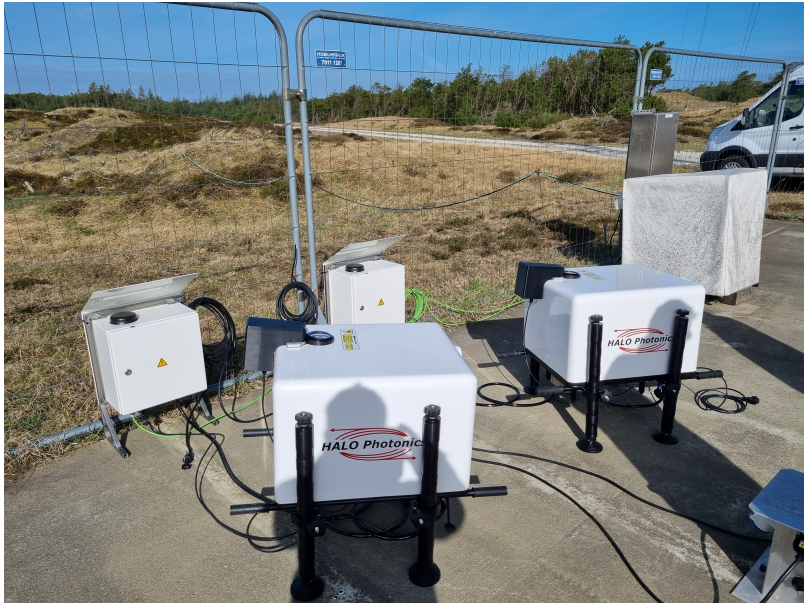
Figure 3. Two BEAM 6x profiling lidars manufactured by Lumibird with serial numbers of 320 and 325, installed during installation at the Østerild test site.
