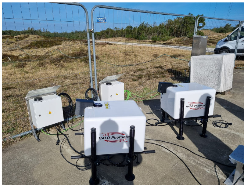
Figure 3. Two BEAM 6x profiling lidars manufactured by Lumibird with serial numbers of 320 and 325, installed at the Østerild test site.
