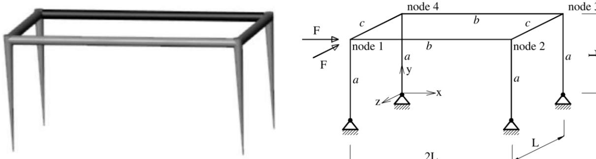
**Figure 1.** Frame displacement at node 13 ([Murín et al. 2002](#))
