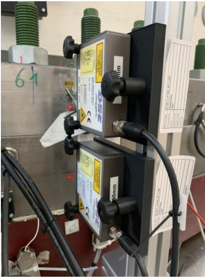
Figure 7: Laser sensors to measure the radial displacement of the outer ring of the lower bearing at 180°
