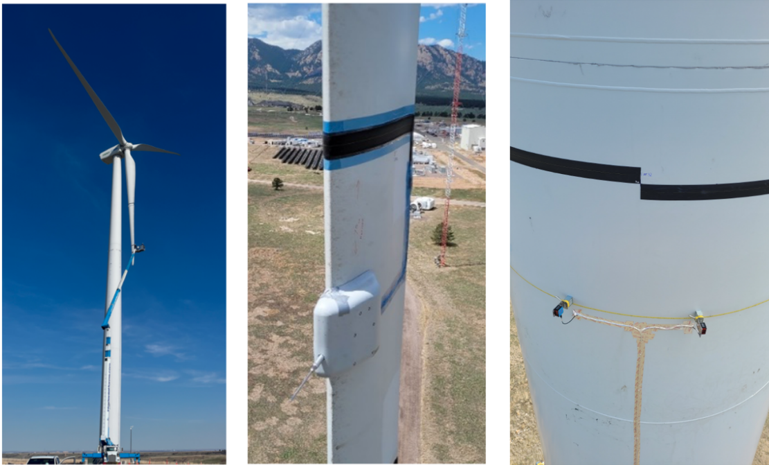
Figure 10. (left) Installation of the outer belt on blade 1 of the GE 1.5 MW wind turbine. The rotor is parked in a downwind configuration. The inner belt and flyboard are visible at the mid-span of blade 1. The belt on the tower had not yet been installed when this photo was taken. Photo credit: Pietro Bortolotti, NREL. (middle) Close-up view of the flyboard, five-hole probe, and belt installed at the outer blade location. Photo credit: Per Hansen, DTU. (right) The belts on the tower, each covering half of the circumference, were installed 1 m above the laser sensors and at the height of the outer belt on blade 1. Photo credit: Per Hansen, DTU.
