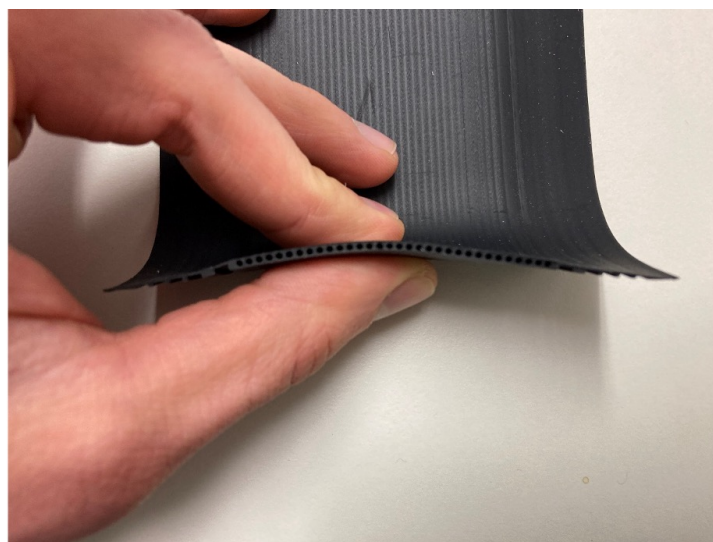
Figure 2. Cross section of the extruded pressure belt. Photo credit: Per Hansen, DTU.
