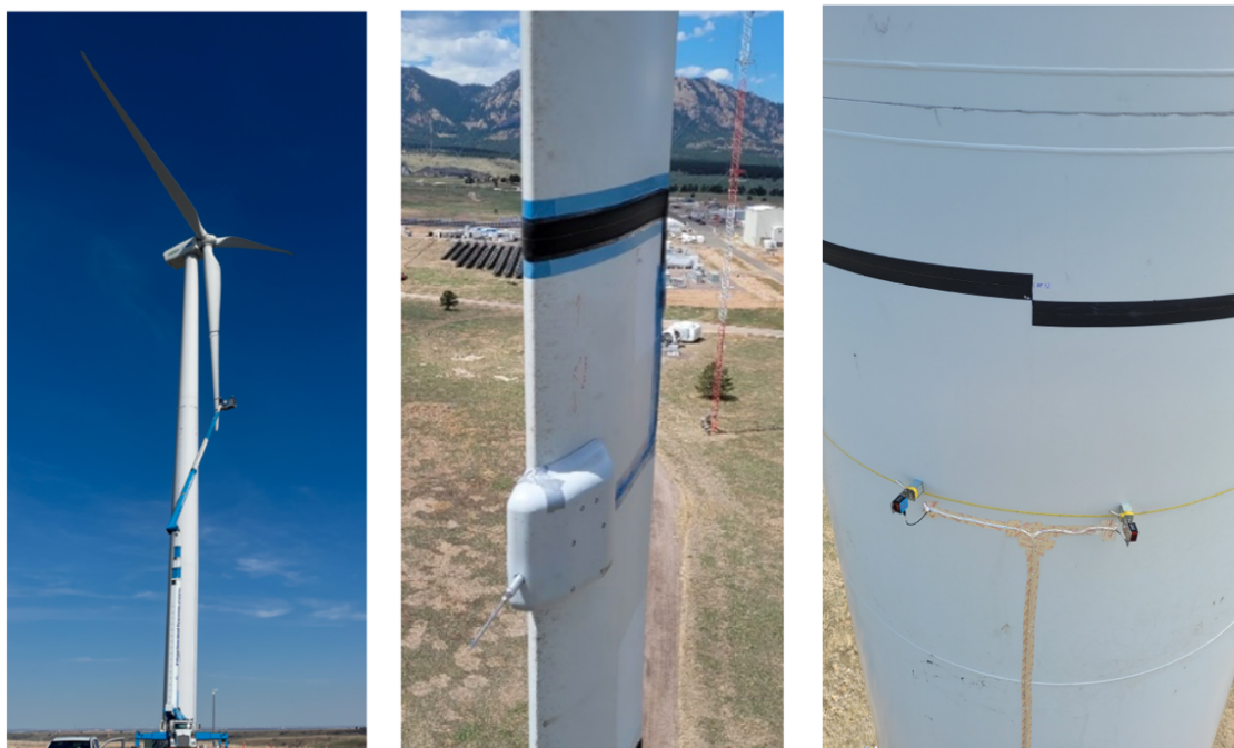
Figure 9. (left) Installation of the outer belt on blade 1 of the GE 1.5 MW wind turbine. The rotor is parked in a downwind configuration. The inner belt and flyboard are visible at the mid-span of blade 1. The belt on the tower had not yet been installed when this photo was taken. Photo credit: Pietro Bortolotti, NREL. (middle) Close-up view of the flyboard, five-hole probe, and belt installed at the outer blade location. Photo credit: Per Hansen, DTU. (right) The belts on the tower, each covering half of the circumference, were installed 1 m above the laser sensors and at the height of the outer belt on blade 1. Photo credit: Per Hansen, DTU.
