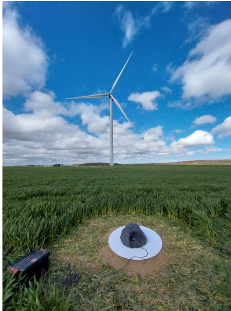
Figure 3. Picture of one SLM with E12 wind turbine in the background. The wheat crops around the SLM were cut to prevent noise disturbance. Following the recommendations of the IEC standard (IEC, 2012), all microphones-SLMs are installed on a woodboard of 1 m diameter and covered by two windscreens.
