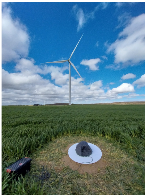
Figure 3. Picture of one SLM with E12 wind turbine in the background. The wheat crops around the SLM were cut to prevent noise disturbance. Following the recommendations of the IEC standard (IEC et al., 2012), all microphones are installed on a woodboard of 1 m diameter and covered by two windscreens.
