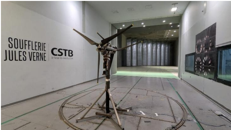
175 Figure 3: The CR-DRWT in the wind tunnel at CSTB.
