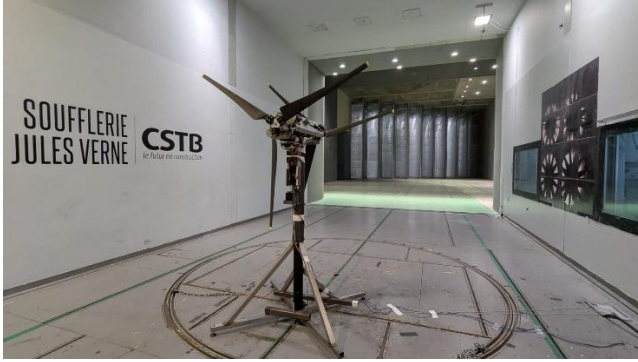
Figure 2: The DRWT in the wind tunnel at CSTB.
