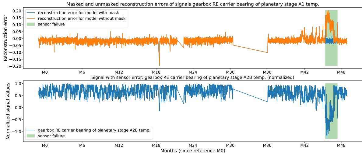
Figure 7. Gearbox RE carrier bearing of planetary stage A2B temperature (bottom plot) sensor failure (bottom plot, green box) and its impact on the reconstruction error of gearbox RE carrier bearing of planetary stage A1 temperature (top plot) without (top plot, orange curve) and with (top plot, blue curve) masking of the sensor error. The data originates from turbine 21 of WF1.
