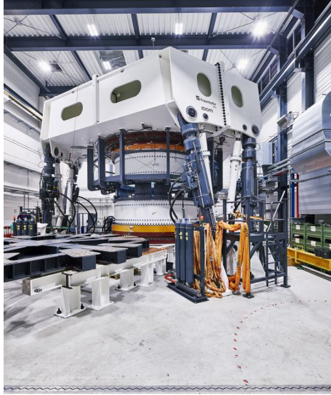
Figure 2. BEAT6.1 test bench ©Fraunhofer IWES/Marcus Heine
