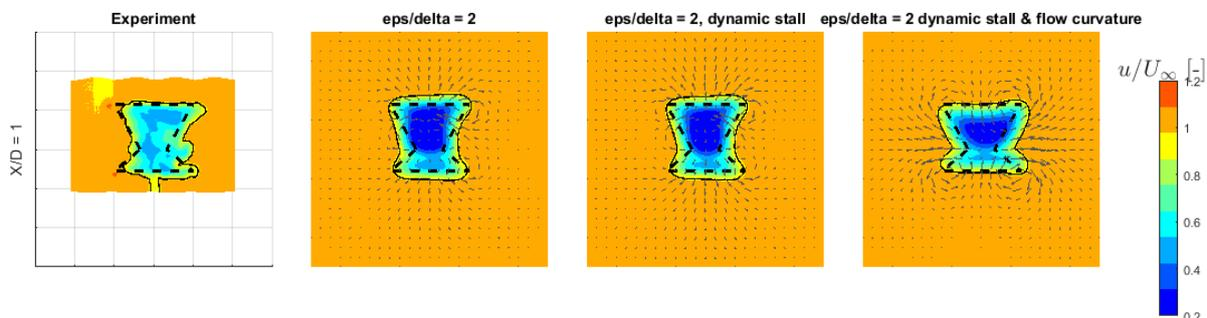
Figure 4: Time-averaged normalised streamwise velocity components for a 1:250th scaled X-Rotor geometry at  $X/D = 1$ .
