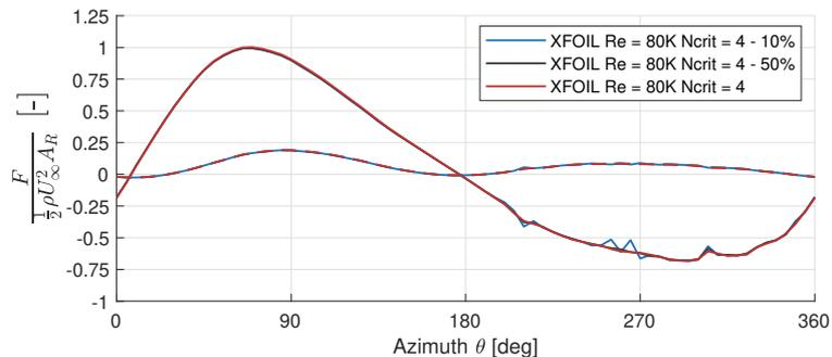
Figure 5: Integrated blade forces  $F$  as a function of azimuth  $\theta$  to show sensitivity to vortex core sizes. The solid lines represent the normal force and tangential force is represented by the dashed lines. Positive normal force is away from the axis of rotation and vice versa. Forces are integrated along both upper and lower halves of B1.
