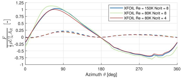
Figure 2: Integrated blade forces  $F$  as a function of azimuth  $\theta$ . The solid lines represent the normal force and tangential force is represented by the dashed lines.
