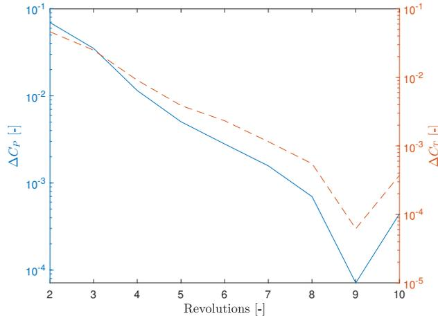
Figure 1: Convergence plot of power and thrust. The Y-axes are in logarithmic scale
