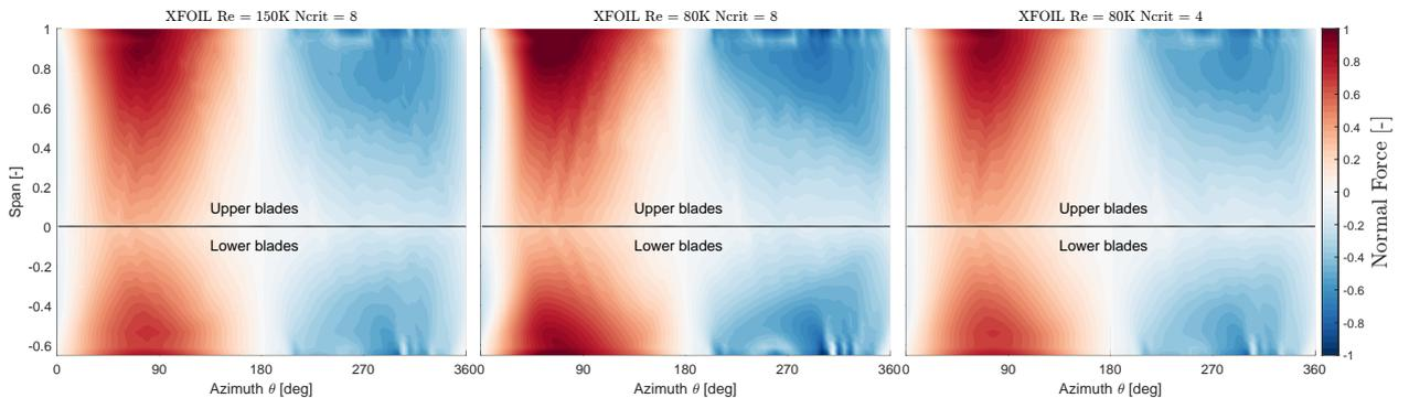
Figure 3: Spanwise distribution of normal blade forces  $F_N$  as a function of azimuth  $\theta$ .
