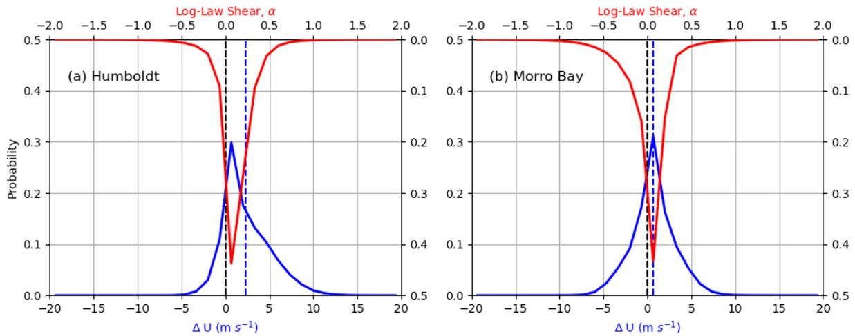
**Figure S10.** Histograms of wind shear expressed as (a) change of wind-speed across rotor-layer ( $\Delta U$ ,  $m s^{-1}$ ; blue) and (b) the log-law shear exponent,  $\alpha$  (red) for Humboldt. Mean value for  $\Delta U$  marked by a dashed blue line.
