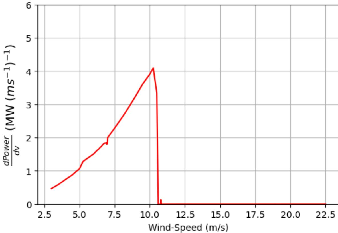
**Figure S13.** Profile of Rate of Change of Power with Wind Speed for the IEA 15 MW Reference Wind Turbine (RWT) with cut-in and cut-off speeds at 3 and 25 m s<sup>-1</sup>, respectively and saturation wind speed of 11.2 m s<sup>-1</sup>.
