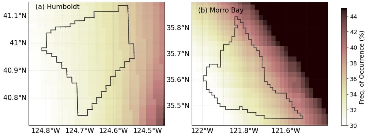
**Figure S8.** Frequency of occurrence of the PBL top heights being less than or equal to the halfway altitude of the wind turbine rotor layers (i.e., PBL top  $\leq$  150 m A.S.L) for (a) Humboldt and (b) Morro Bay wind energy lease areas.
