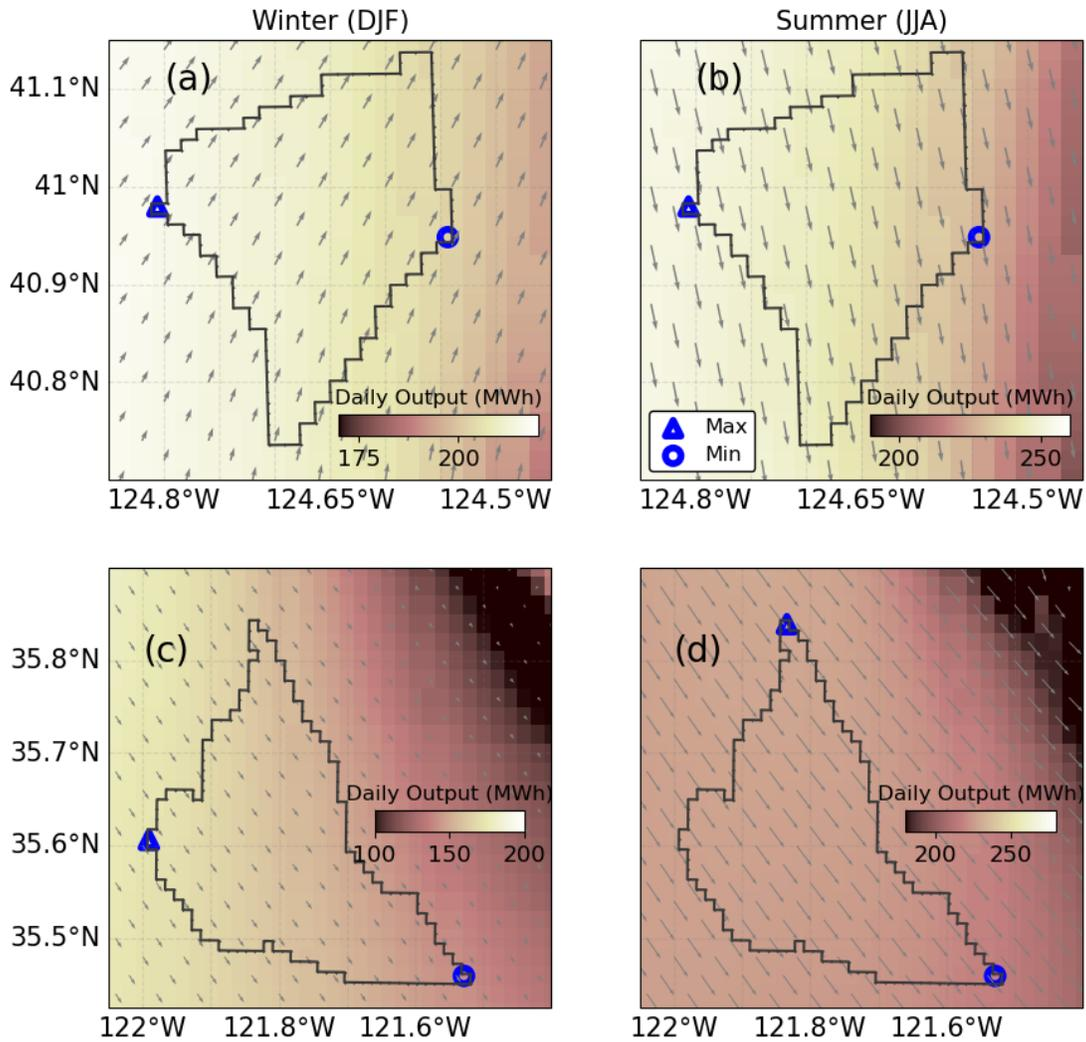
**Figure S2.** Seasonally Averaged daily energy output (colors), hub-height wind speeds (arrows), and the locations of the grid-cells with maximum (MAX) and minimum (MIN) overall energy output for the (a, b) Humboldt and (c, d) Morro Bay WEAs. Left panels show mean values for winter months (DJF) and right panels show mean values for summer months (JJA).
