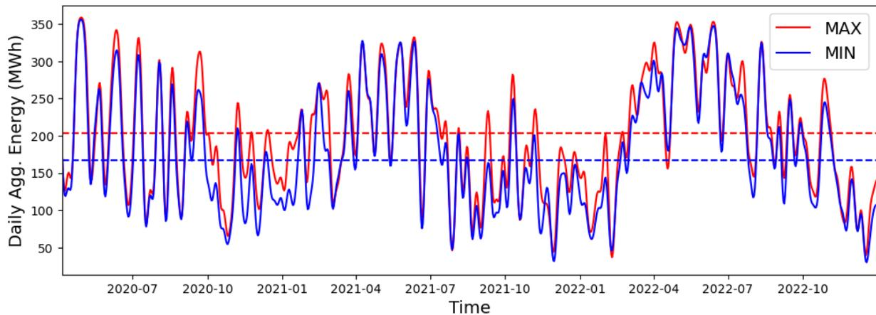
**Figure S6.** Time series of Daily Aggregate Energy Output for the points of MAX energy output (red) and MIN energy output (blue) for Morro Bay. Overall mean energy output for both points are shown in dashed lines of the corresponding color.
