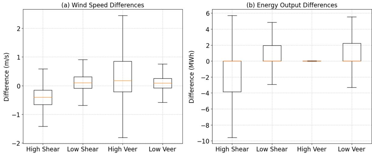
**Figure S12.** Histograms of difference between (a) hub-height and equivalent wind-speeds and (b) energy outputs computed for the hub-height and equivalent wind-speeds, at Humboldt Bay for regimes of high shear and high veer. Shown values are the hourly estimates from all grid cells within the respective WEAs.
