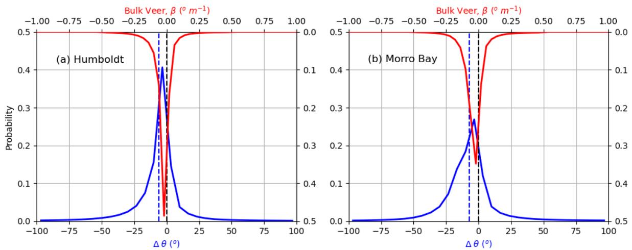
**Figure S11.** Histograms of wind veer expressed as (a) change of wind-direction across rotor-layer ( $\Delta \theta$ ,  $^{\circ}$ ; blue) and (b) the bulk veer exponent,  $\beta$  (red) for Humboldt. Mean value for  $\Delta \theta$  marked by a dashed blue line.
