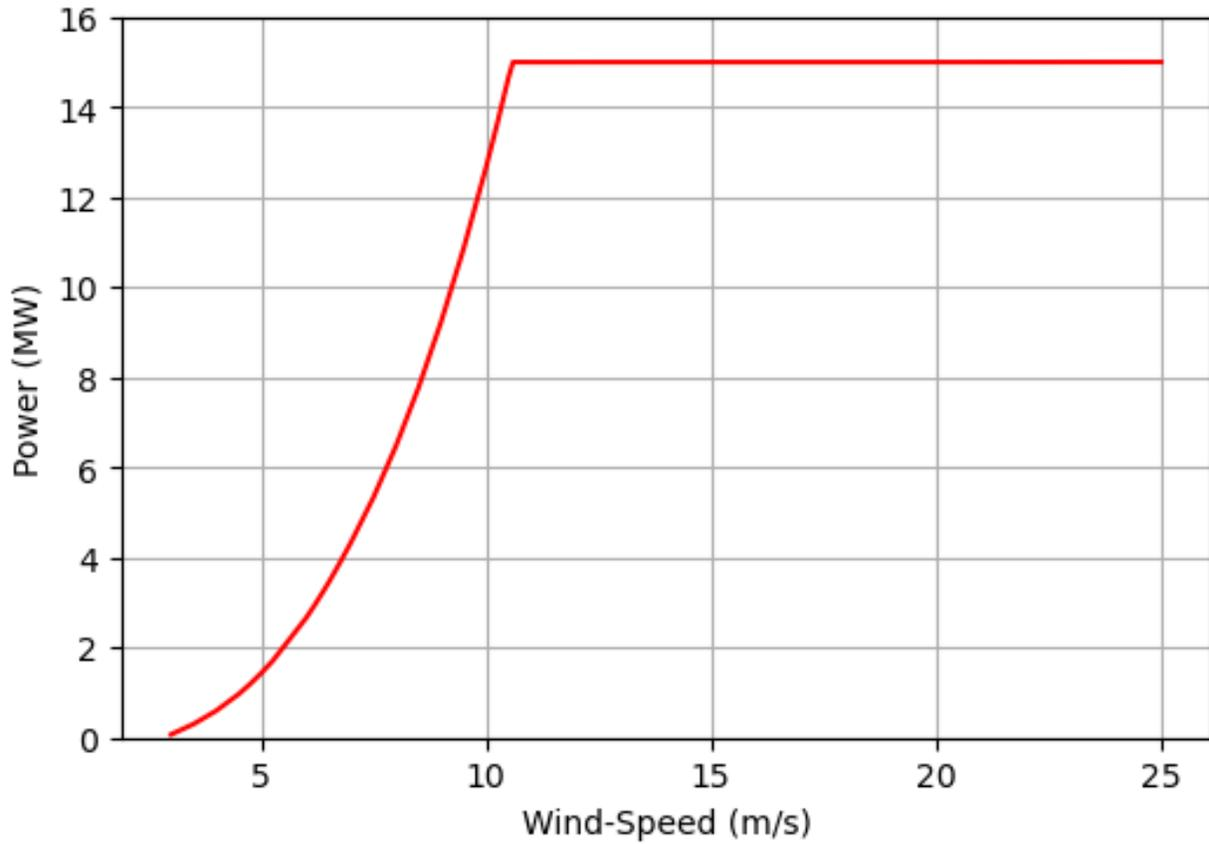
**Figure S1.** Power Curve for the IEA 15 MW Reference Wind Turbine (RWT) with cut-in and cut-off speeds at 3 and 25 m s<sup>-1</sup>, respectively, and saturation wind speed of 11.2 m s<sup>-1</sup>.
