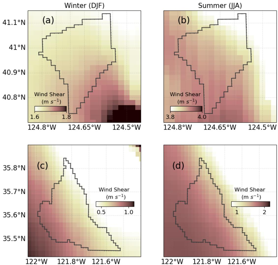
**Figure S7.** Seasonal mean rotor-layer wind shear ( $\text{m s}^{-1}$ ) at the Humboldt Bay wind energy lease area (top panels) and Morro Bay wind energy lease area (bottom panels). Panels (a) and (b) show wind shear for winter (DJF) and summer (JJA) at Humboldt, while panels (c) and (d) show wind shear for winter and summer at Morro Bay.
