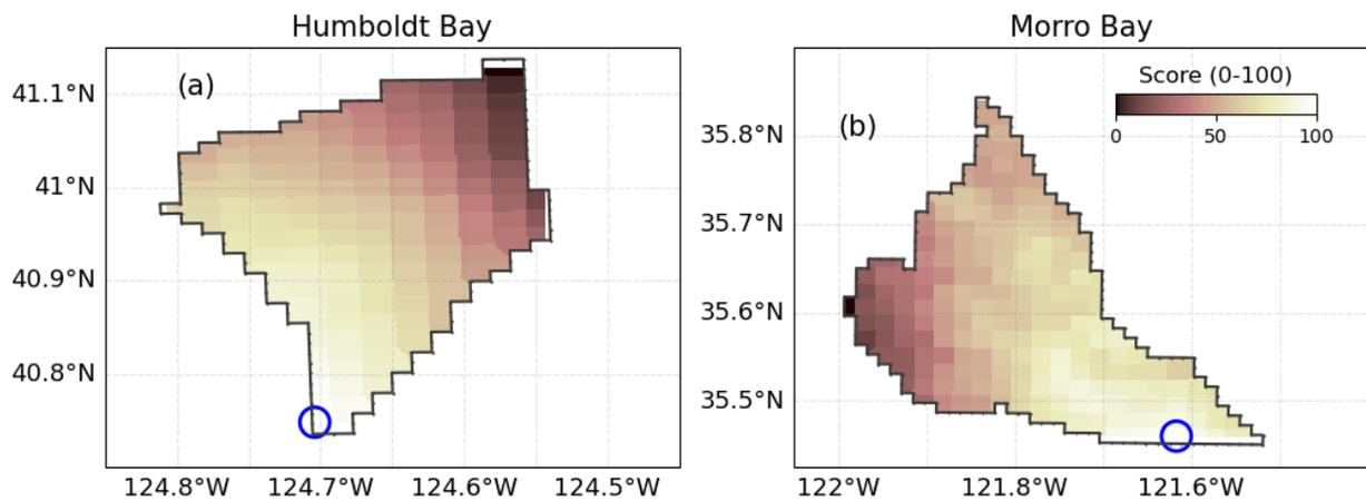
**Figure S18.** Mean Linear Optimization Score for grid cells at (a) Humboldt and (b) Morro Bay (brown) wind energy lease areas after optimizing for all 25 randomly generated power curves of Figure S10. The locations of the most optimal wind resource (MAX Score) at each wind energy lease area are marked with a blue circle. Note that in this case, the scores can lie anywhere between 0 and 100, but not necessarily exactly covering that range.
