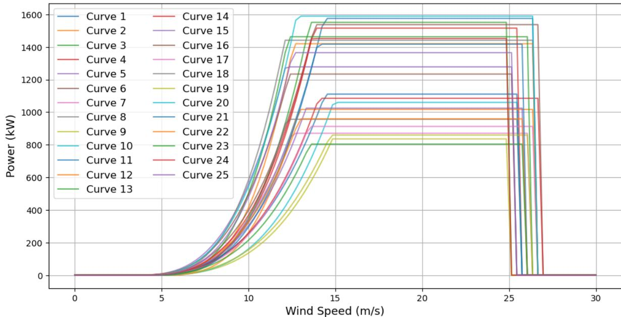
**Figure S17.** 25 Randomly Generated Wind Turbine power curves between rated powers of 8-16 MW, derived by choosing random values of cut-in and cut-out wind speeds and rated wind speeds and powers.
