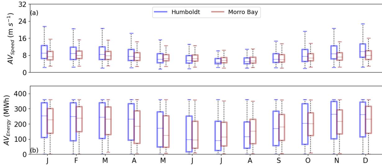
**Figure S15.** Monthly variation of absolute variability (AV) of (a) Hub-height (150 m A.S.L) wind speeds, (b) Power (MW), and (c) Planetary Boundary Heights (km) at Humboldt (blue) and Morro Bay (brown) wind energy lease areas.
